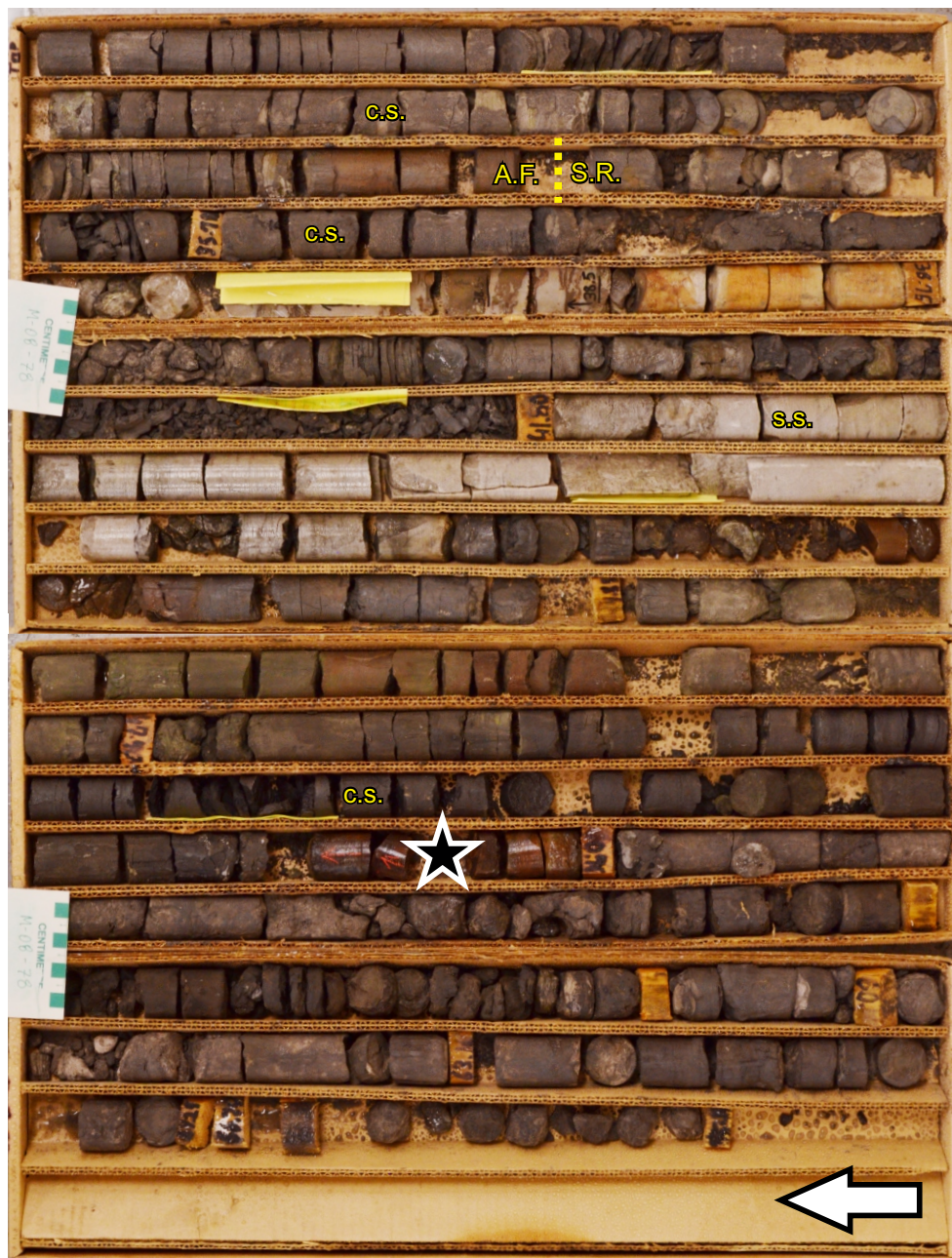
Figure GS2019-7-2: Photograph of the Swan River Formation in drillcore M-08-78 (Bannatyne, 1978). Lowermost shale beds of the Ashville Formation occur near the top of the interval, underlain by sandstones and carbonaceous shales of the Swan River Formation. Arrow indicates up direction in core. Scale bar in centimetres. Star denotes location of the fossilized leaf-bearing nodule. Yellow dashed line denotes contact between Ashville and Swan River formations. Abbreviations: A.F, Ashville Formation; c.s., carbonaceous shale; S.R., Swan River Formation; s.s., sandstone.
