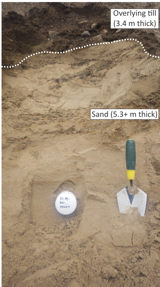
Figure GS2019-9-5: Example of sub till medium sand at section 112-19-621. This sediment was sampled to determine its age using optically stimulated luminescence dating methods. Dashed white line denotes contact between sediments.
