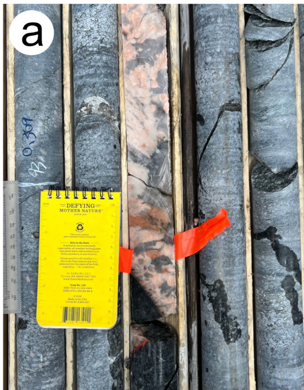
Figure GS2023-4-5: Samples from drillhole LT-21-11: a) contact of a dike composed primarily of quartz and feldspar at 45 degrees to the core axis (95.8 m depth); b) green spodumene within a white dike (48.1 m depth). All core pictured is NQ (47.6 mm diameter).
