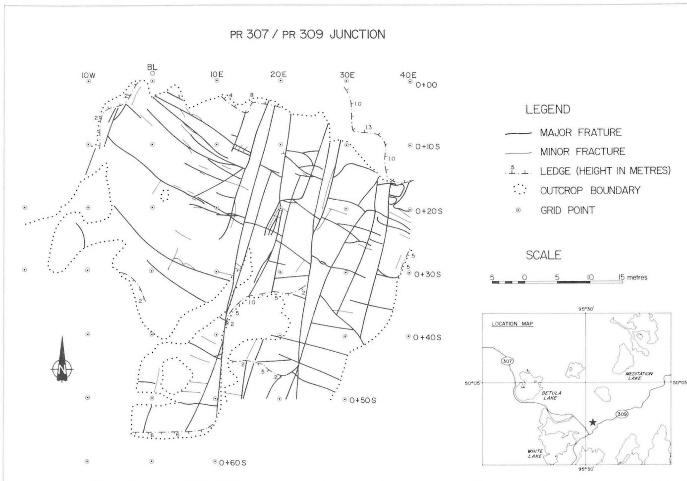
Figure GS-25-8: Joint diagram of pink porphyritic granite of the Betula Lake Pluton.
