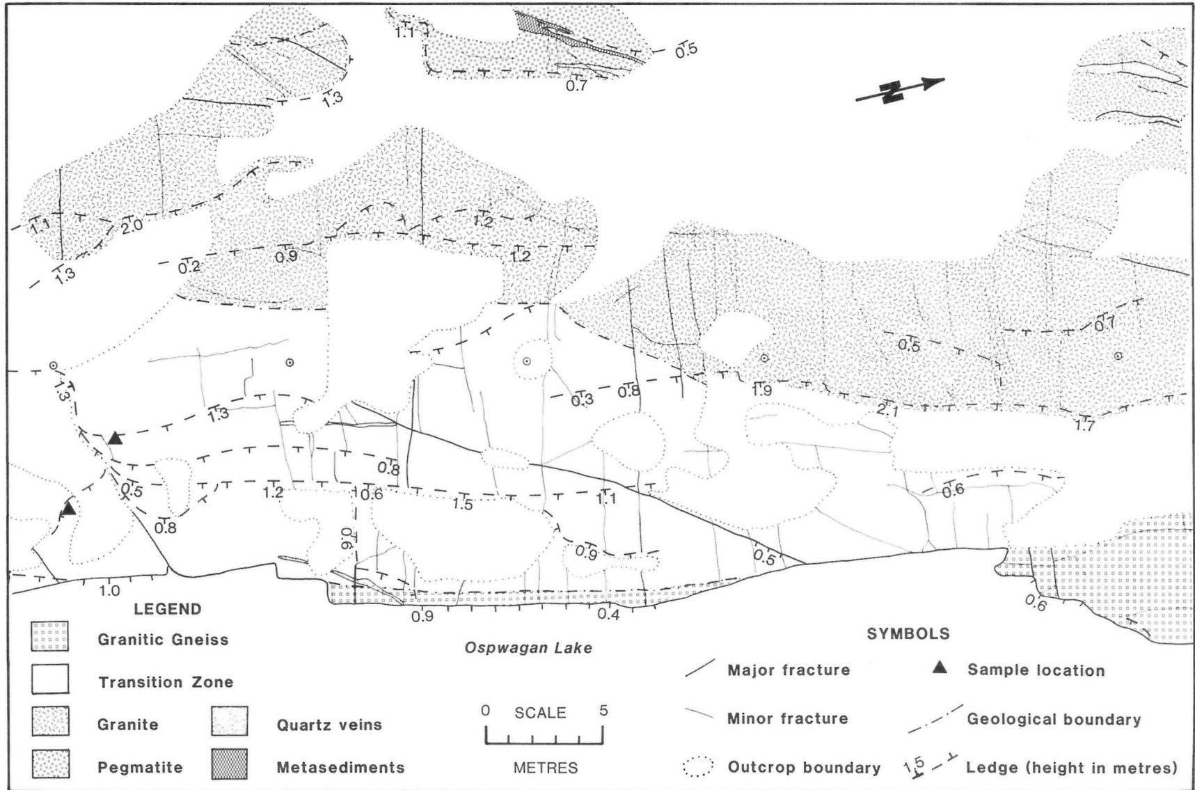
Figure GS-17-7: Detailed structural and lithological map of Oswagan granite.
