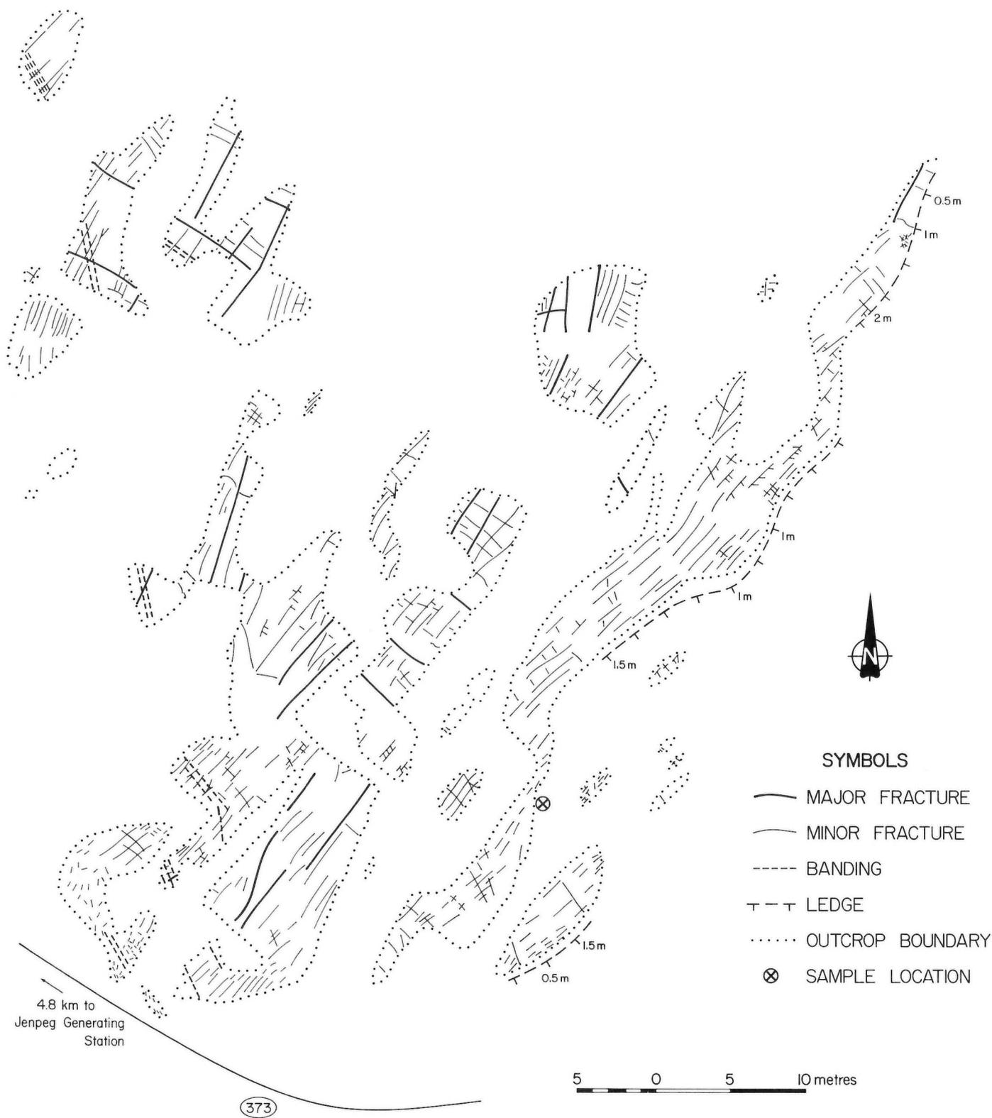
Figure GS-17-8: Detailed structural map of the Cross Lake diabase.
