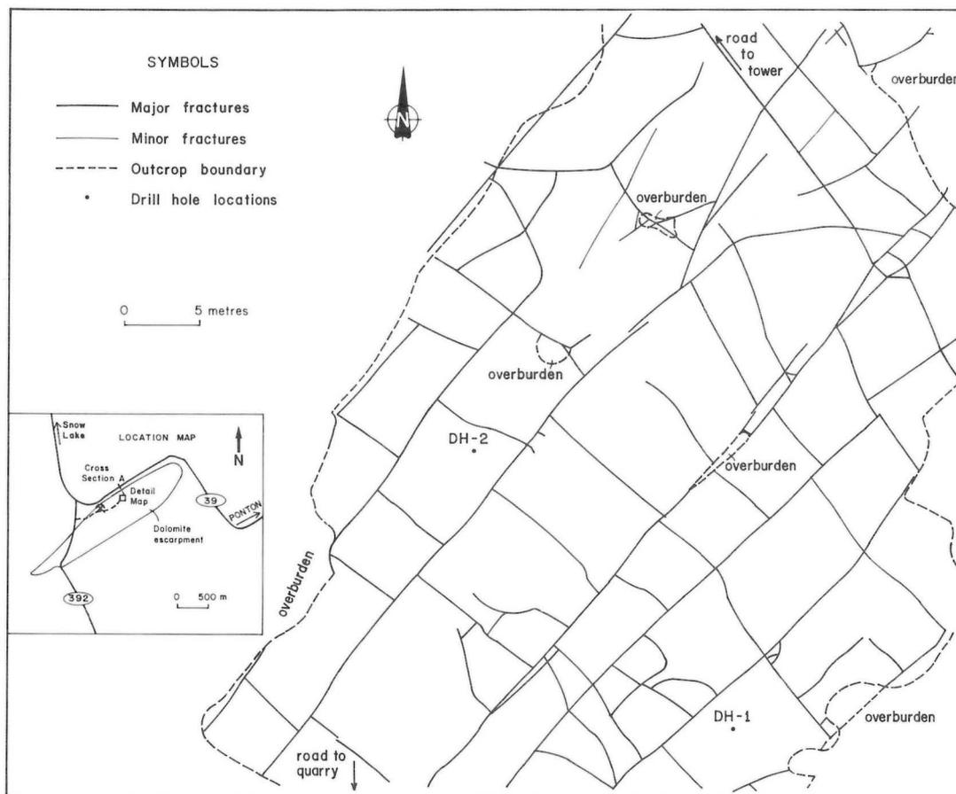
Figure GS-17-4: Wekusko dolomite: joint map.
