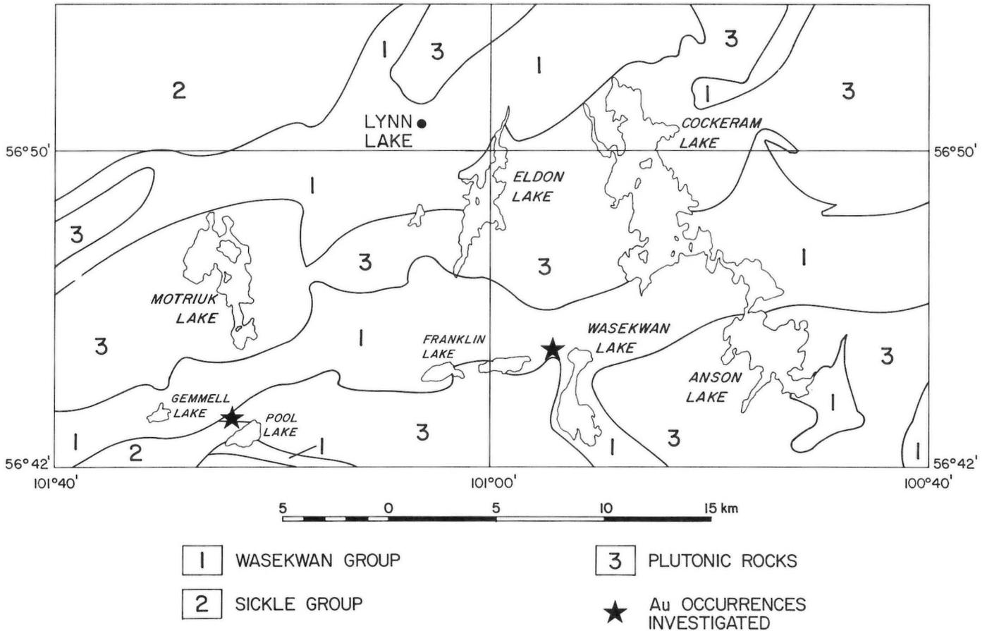
Figure GS-1-1: Location of areas of investigation on the Johnson Shear Zone (\*) and general geology of the Lynn Lake area.
