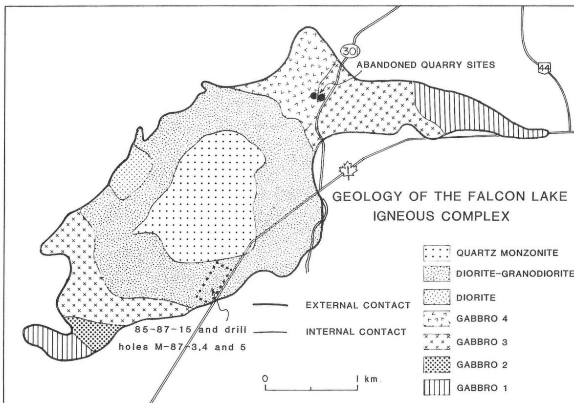
Figure GS-25-3: Geology of the Falcon Lake Igneous Complex and location of outcrop studied for dimension stone potential in 1987. (After Mandziuk et al. 1986).
