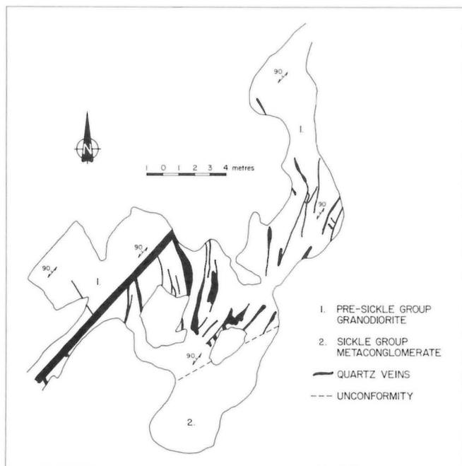
Figure GS-1-3: Outcrop map of sulphide and gold occurrence in quartz vein in pre-Sickle Group granodiorite in the Gemmell Lake area.
