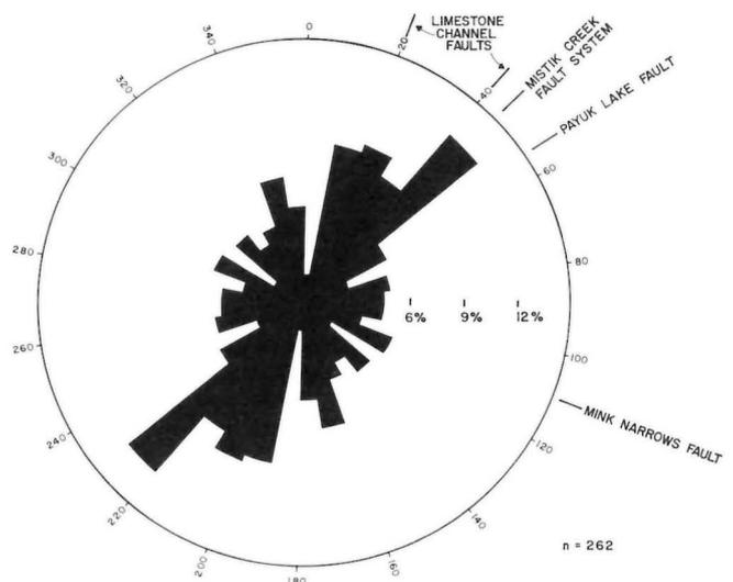
Figure GS-7-9: Rose diagram showing orientations of shear zones, fractures and veins in the area bounded by Mistik Creek fault, Limestone Channel fault, and Mink Narrows fault.
