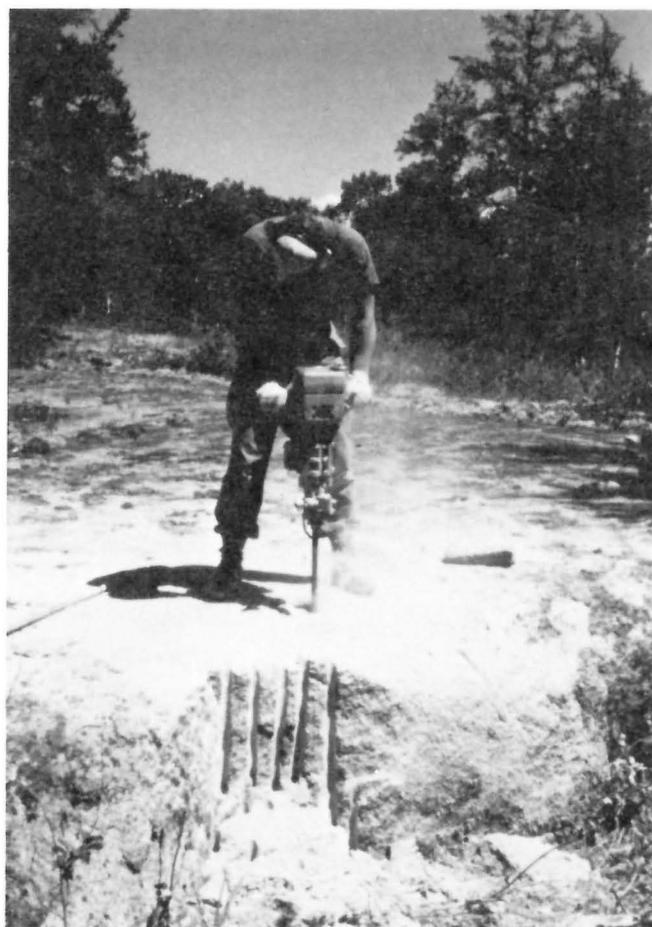
Figure GS-25-2: Porphyritic granite sampled with a Cobra drill and feather and wedge set.
