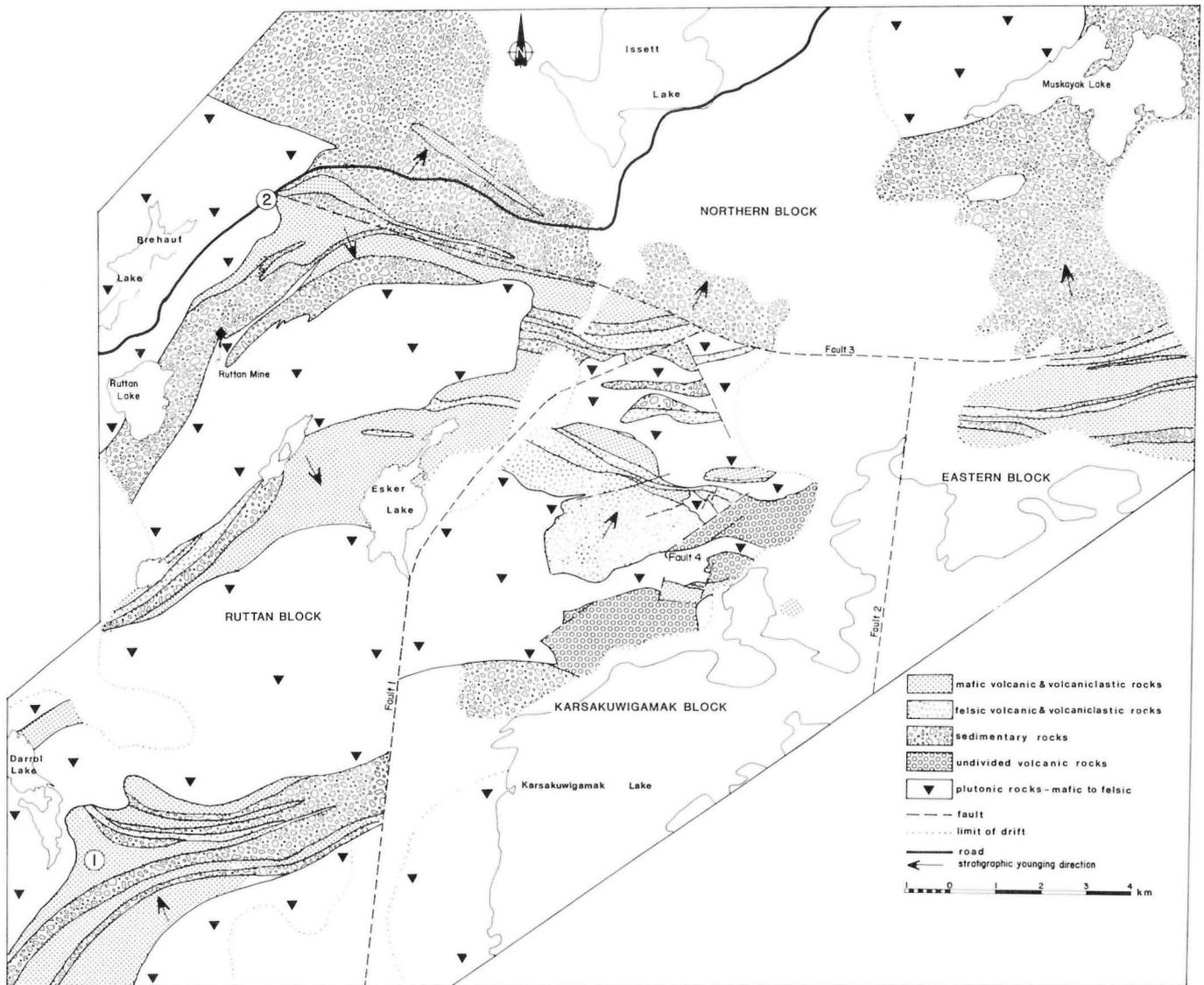
Figure GS-5-1: Geology of the southern part of the Rusty Lake metavolcanic belt and the location of the Darrol Lake iron formation (1) and the Vol deposit (2).
