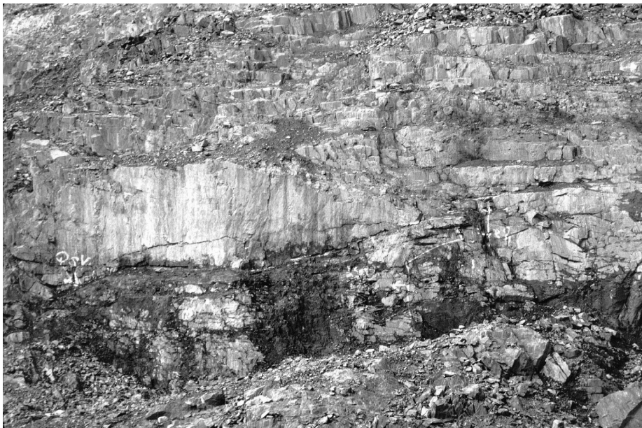
Figure GS-16-3: Quartz-sulphide vein (QSV) along southwest-dipping fault, East Pit, Farley Lake Deposit. Looking north. Field of view ~10 m.
