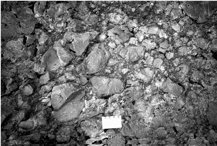
Figure GS-14-18: Pillow fragment breccia, flow 15, Jackfish Falls, Upper volcanic formation. Fragments are equant and angular, some preserving pillow selvages. This type of breccia is rare in the exposed volcanic section and may be related to a nearby synvolcanic fault (Fig. GS-14-2).
