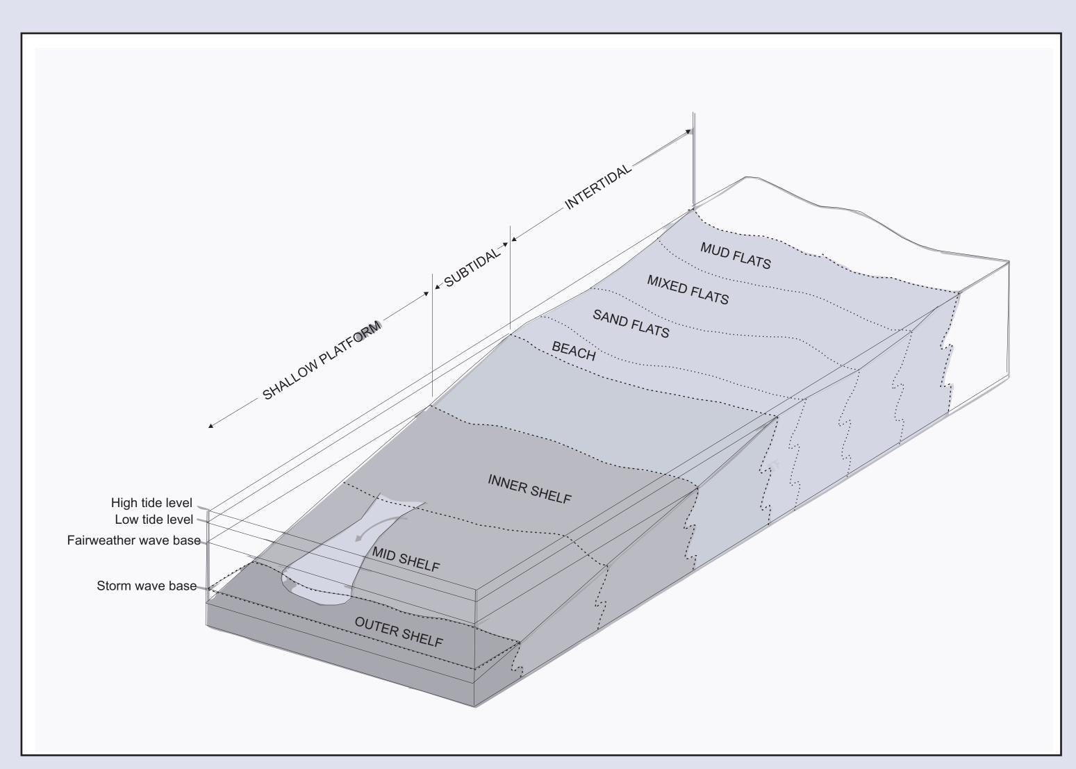
Figure 5: Schematic diagram displaying the distribution of Three Forks facies along an unrimmed carbonate platform and high-energy carbonate tidal flat. (Karasinski, 2006)
