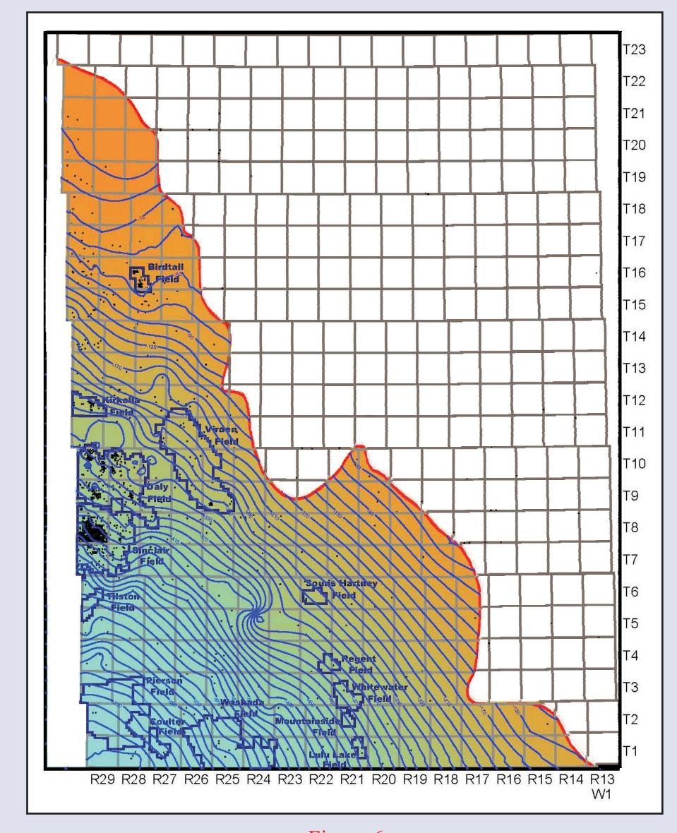
Figure 6 Devonian Three Forks Formation: Structure Contour Contour Interval =20 m
