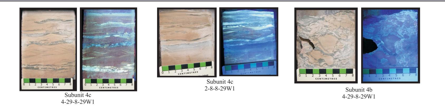
Figure 4: Core photos of Sinclair reservoir subunits 4b and 4c taken in white (left) and ultraviolet (right) light. Yellow fluorescence is oil, and blue fluorescence is anhydrite.
