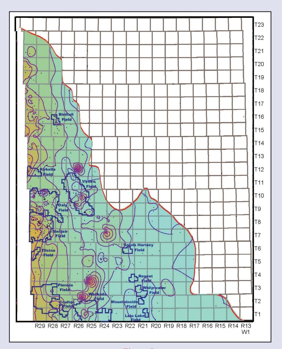
Figure 8 Devonian Three Forks Formation: Isopach Contour Interval =5 m
