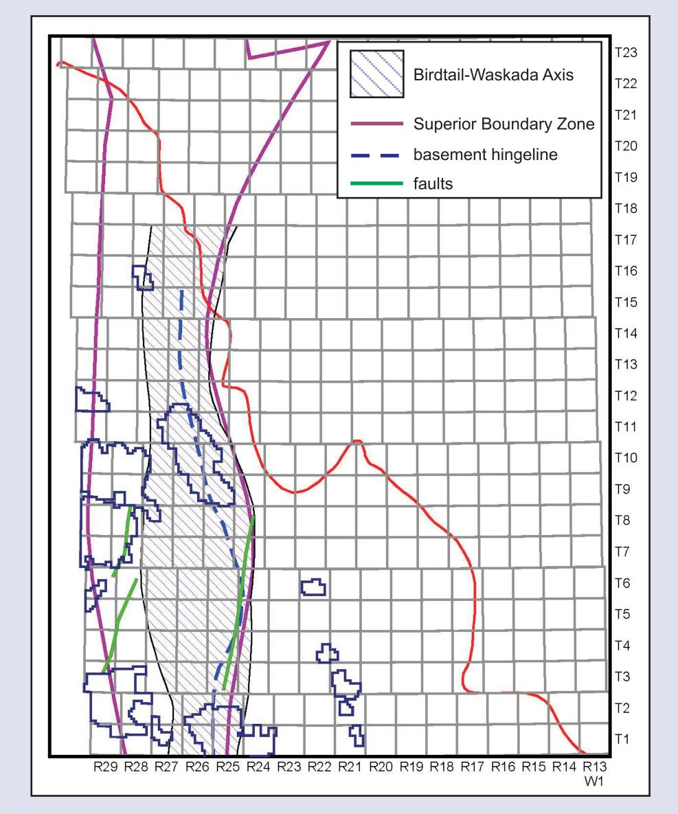
Figure 10: Tectonic map showing postulated fault lines.
