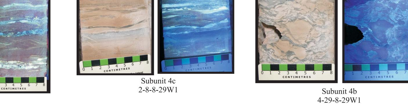
Figure 4: Core photos of Sinclair reservoir subunits 4b and 4c taken in white (left) and ultraviolet (right) light. Yellow fluorescence is oil, and blue fluorescence is anhydrite.
