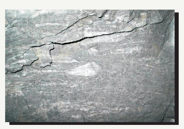
Dark grey massive mineralization (QCMS) including boudinaged quartz veins parallel to the composite S<sub>1</sub>/S<sub>2</sub> transposition foliation.
