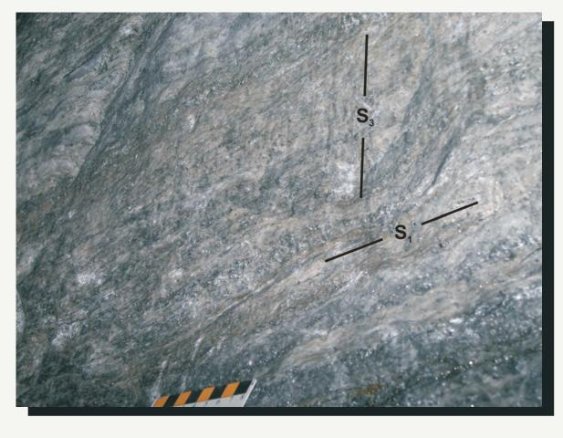
Weak S<sub>3</sub> foliation developed in mineralized sericite schist in the 2 Zone 5 South lower stope.
