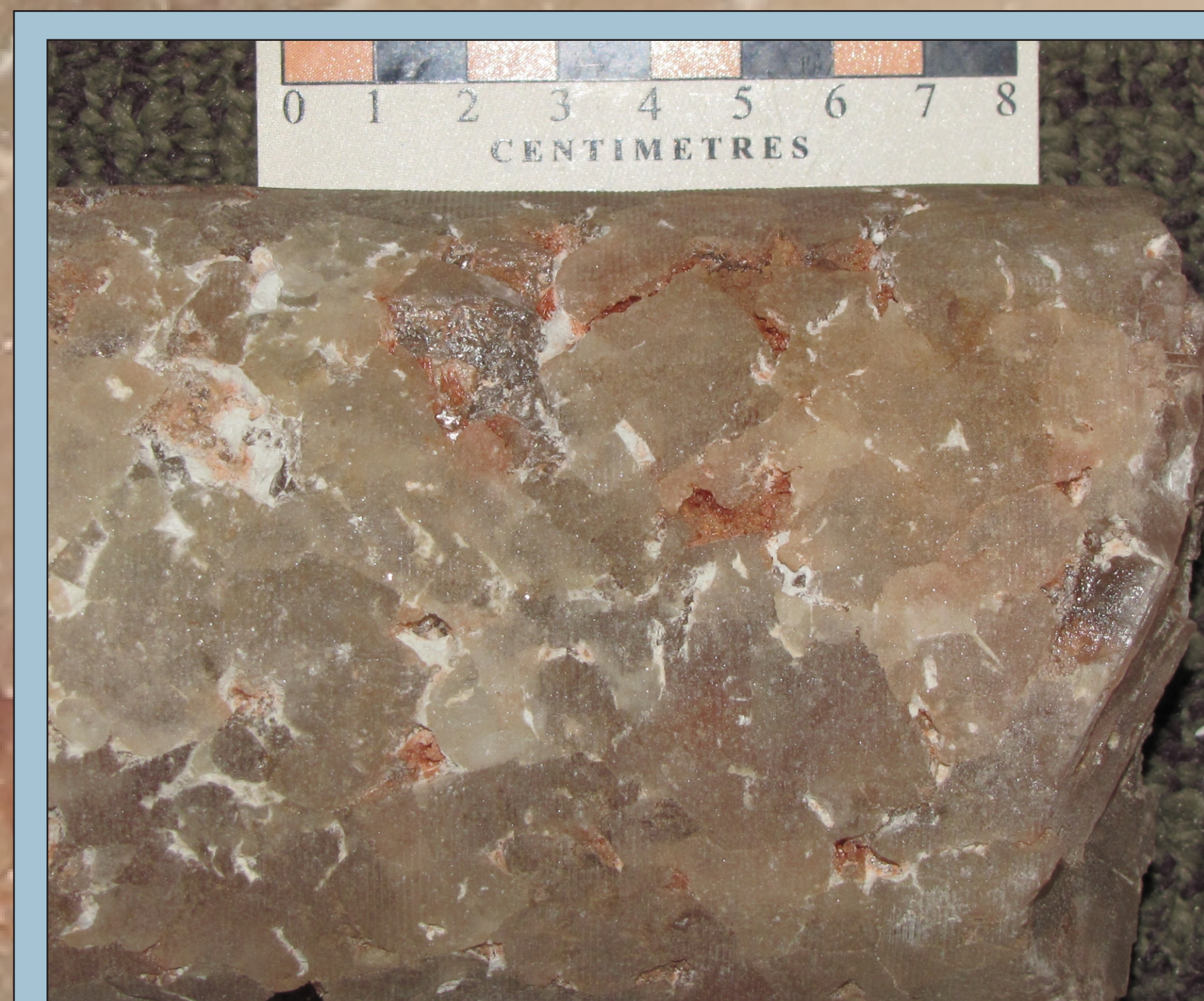
Figure 7: Core photograph of the Esterhazy Member, Prairie Evaporite, showing the potash ore from an approximate depth of 970 m at 8-6-17-29W1.
