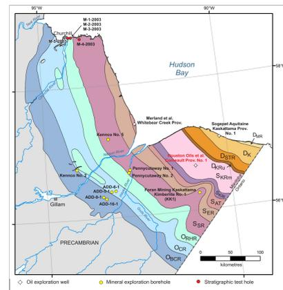
**Figure 5:** Stratigraphic map of the Hudson Bay Lowland, showing location of oil exploration wells, mineral exploration boreholes and stratigraphic test holes. See Figure 1 for legend. (From Nicolas et al., 2014)
