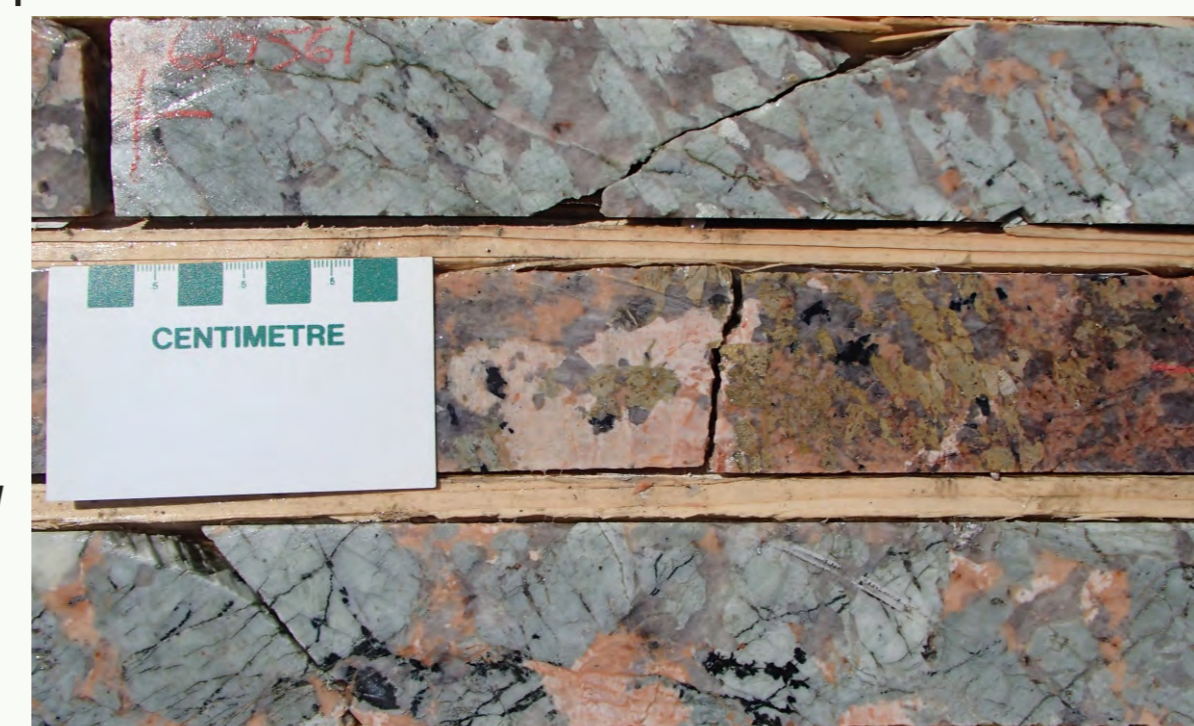
Photo of halved drill core of Dike 1 showing abundant spodumene (green mineral).
