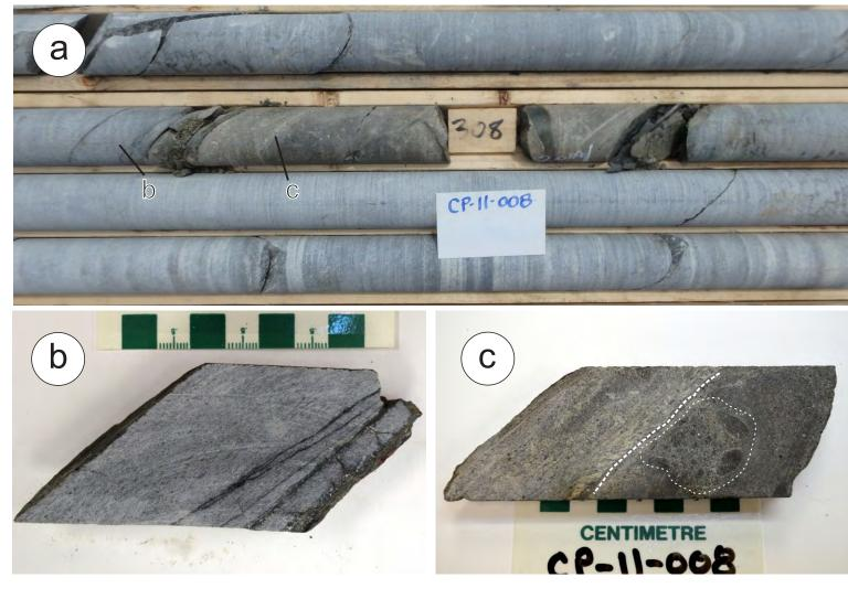
Drillcore photos of intrusive dike CP-11-008: a) brownish-grey intrusive rock with sharp contacts, 307.75-308.10 m; b) sharp contact between felsic lapilli tuff and the intrusive rock, 307.70 307.75 m; c) internal structural heterogeneity of the intrusive rock, defined by layers rich in dolomite segregations, phlogopite macrocrysts and xenoliths, 307.75-307.90 m.
