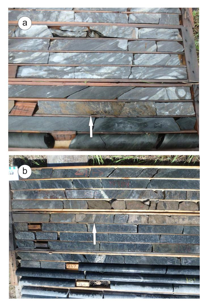
Drillcore photos: a) brecciated and dismembered smoky grey guartz in mafic wacke - net textured pyrrohotite (arrow) along the margin contains 0.41 g/t Au over 194-195.08 m, HAR-181, 194.0m, b) Au-bearing semi-massive pyrrohotite (arrow), KUS368, 249.0-252.0 m.
