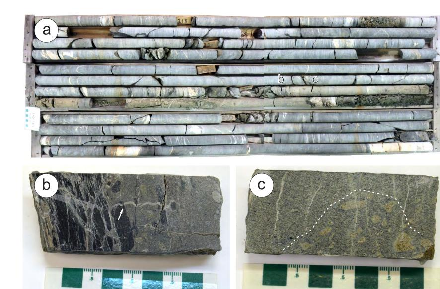
Drillcore photos of intrusive dike KUS303: a) main intrusive intercept (227-229 m); b) gradation from clast-supported to matrix-supported breccia at the intrusive rock contact – arrow points to a late-stage carbonate-filled vein, 227.0 m; c) locally concentrated phlogopite macrocrysts (outlined by dashed line), 227.10 m.
