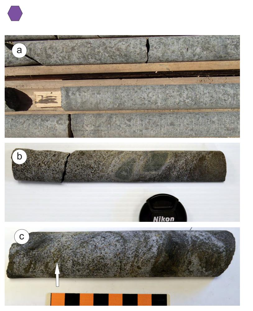
Drillcore photos of gabbro: a) coarse grained gabbro from west of the Blackduck Ni-Cu deposit FARE-8, 236 m; b) mela-gabbro with andesite xenoliths, 138-24 163.0m; c) mela-gabbro with disseminated sulphides (arrow), 138-24, 165.0 m.
