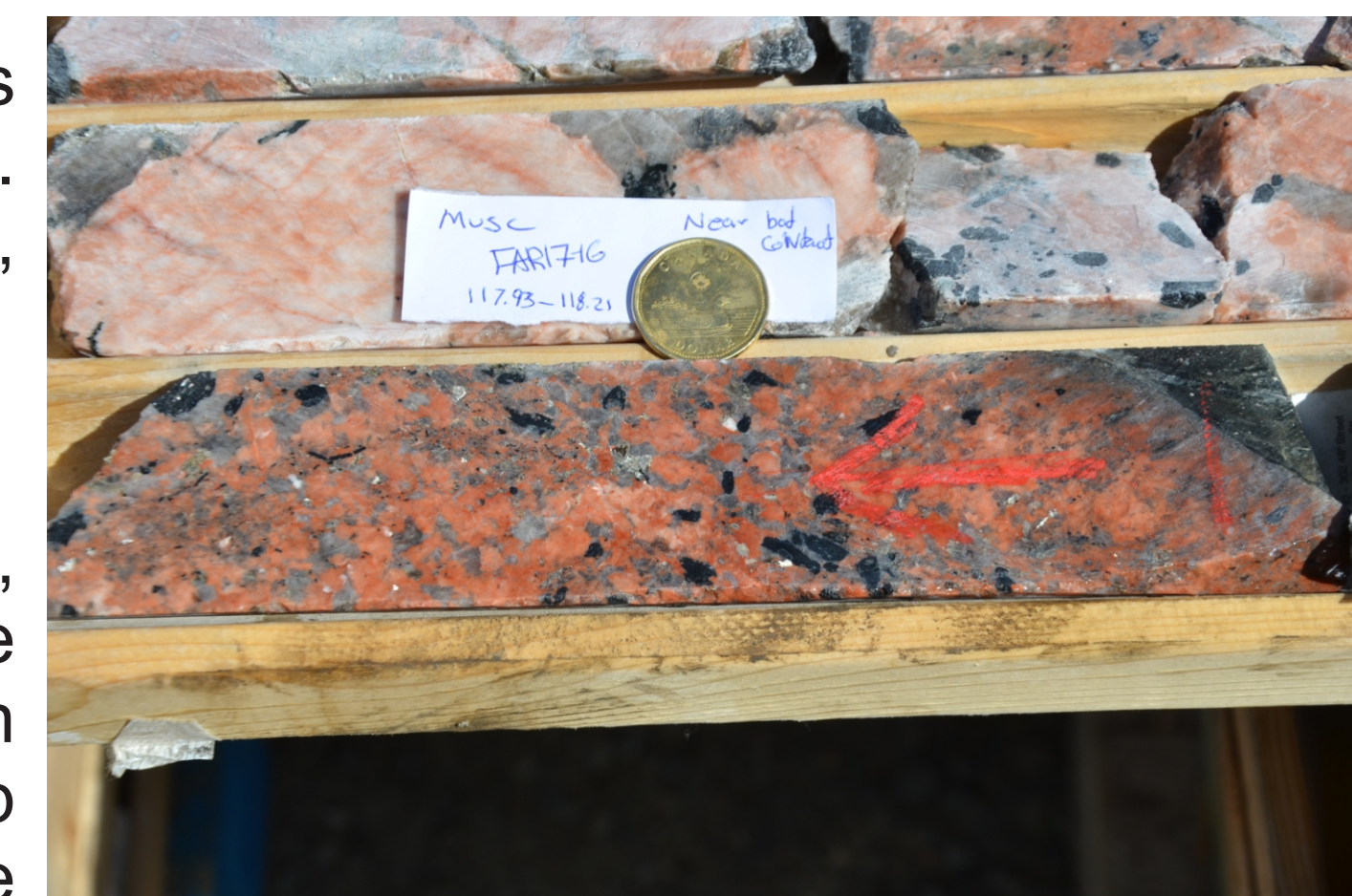
Figure 3: Drillcore sample displaying the brick red colour of the wall zone, coin for scale.
