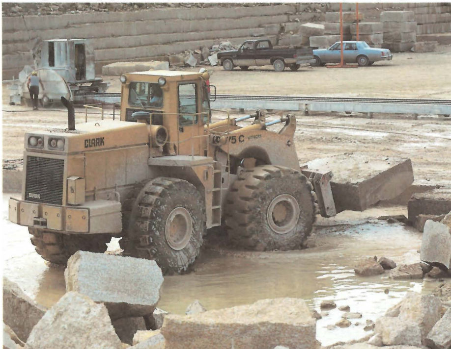
Extracting cut block of Tyndall Stone for transportation to the finishing plant, Gillis Quarry, Garson.
