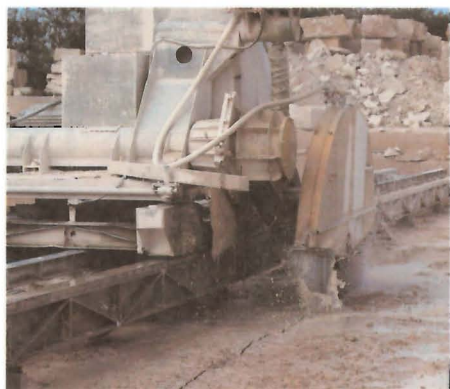
Above: Extraction of Tyndall Stone at the Gillis Quarry, using a circular rock saw.
