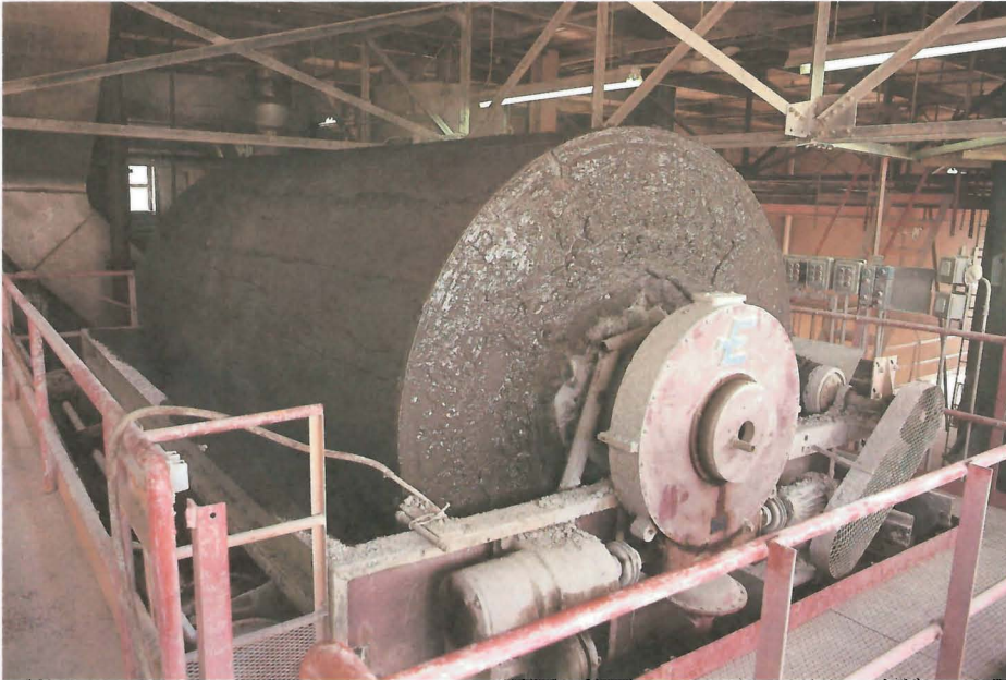
Bentonite dryer, after acid treatment, Pembina Mountain clays, Winnipeg.
