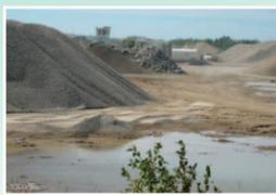
Gravel pit showing stockpiles of different sizes of gravel. Sand and gravel from the pit is put through a machine called a screener, which sorts the material into the different sizes.
