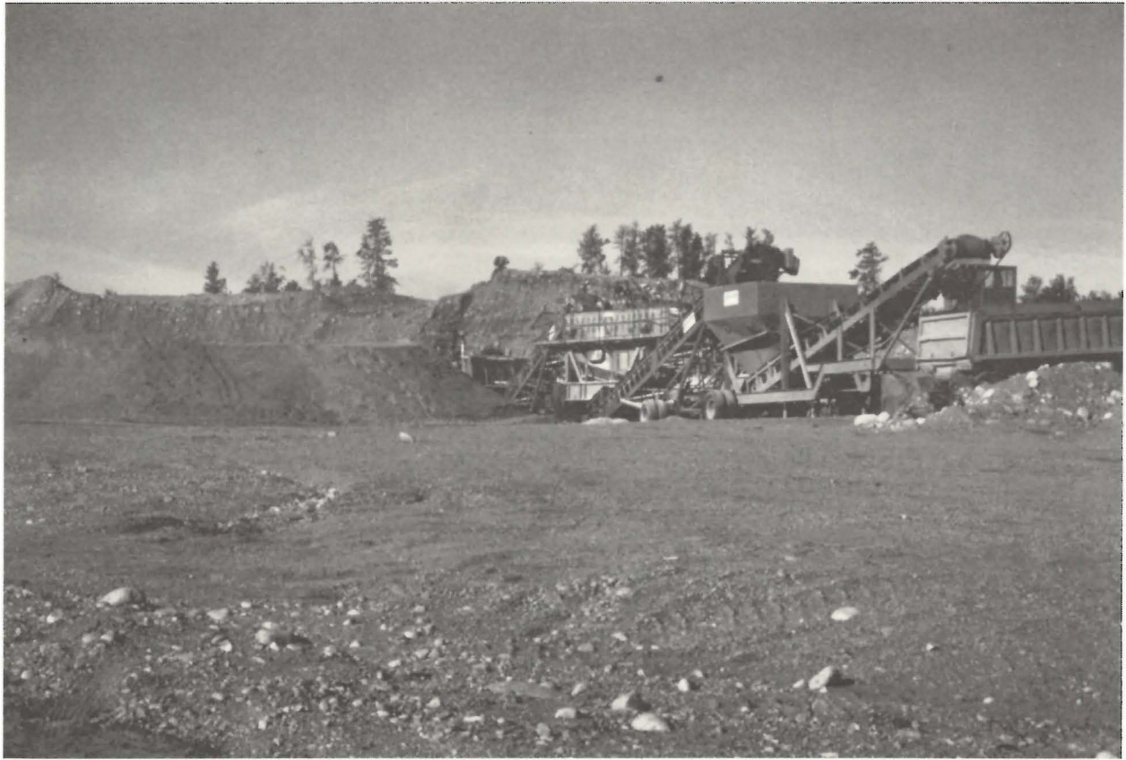
Photo 3. Portable screening-crushing plant at Leaf Rapids.
