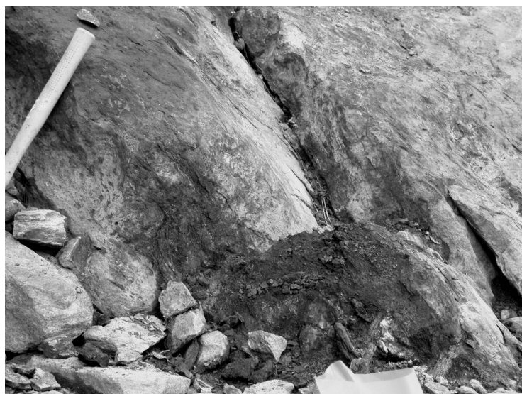
Figure 28: Semimassive Fe-sulphide-graphite occurrence with trace chalcopyrite, Rat Lake region, NTS 64B (Uhlman Lake).
