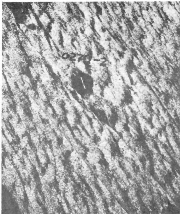
Plate 4-1. Typical blotchy weathered surface and intersecting foliations in unit 5.
