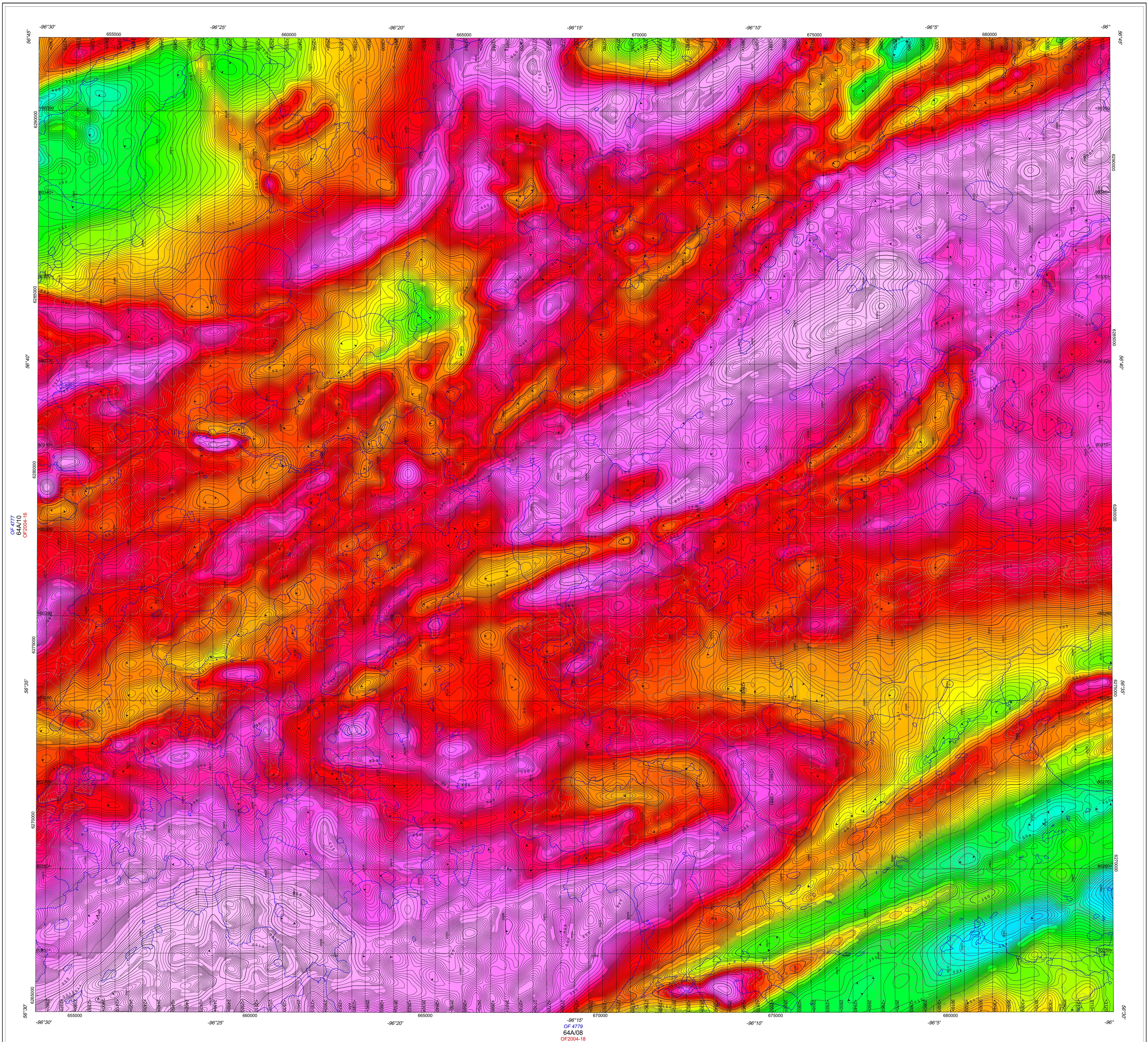
This map was compiled from data obtained as a result of an aeromagnetic survey carried out by Goldak Exploration Limited using a Piper PA-31 Navajo (registration C-GJBB) aircraft. A 0.005 nT interval split-beam cesium vapour magnetometer was mounted in the tail boom of the survey aircraft.
