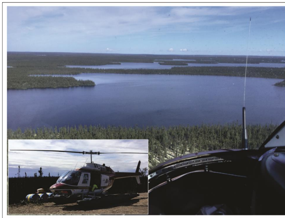
Figure 6 A Bell 206B (Jet Ranger) helicopter on floats (inset) on approach to a typical lake (1 to 5 km 2 ) for sampling. Pre-labelled synthetic cloth bags and high-density polyethylene (HDPE) bottles are used to collect (approximately) a 1-kg sample of lake sediment and a 250-ml sample of surface lake water.
