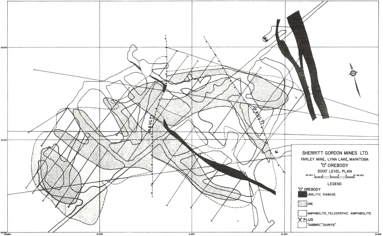
NM 7504-B Figure 4 A geological plan of the 2000' level in the "O" orebody of the Farley Mine, Lynn Lake; geology after Sherritt Gordon Mines Limited.
