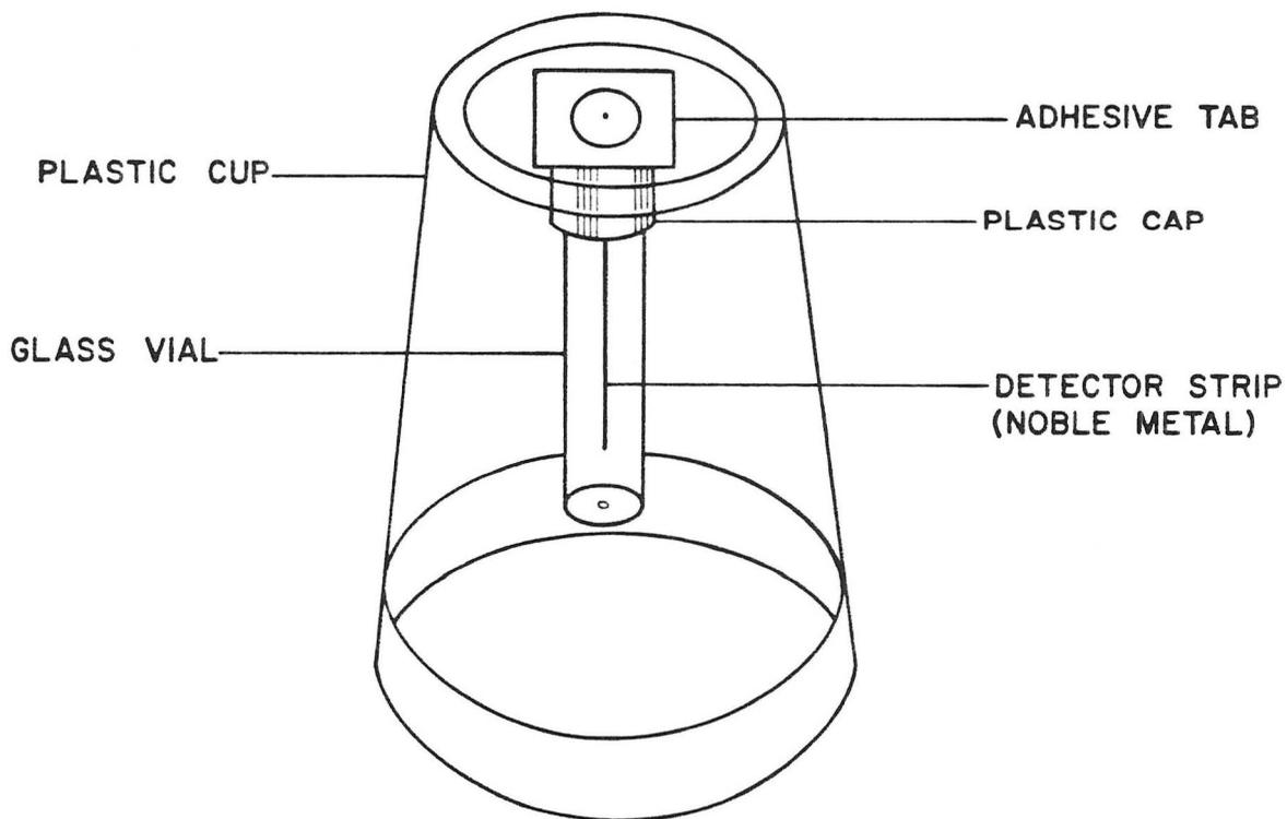
Figure 3: Components of an Aurex Cup. Diagram from Earth Search Inc., 1985.
