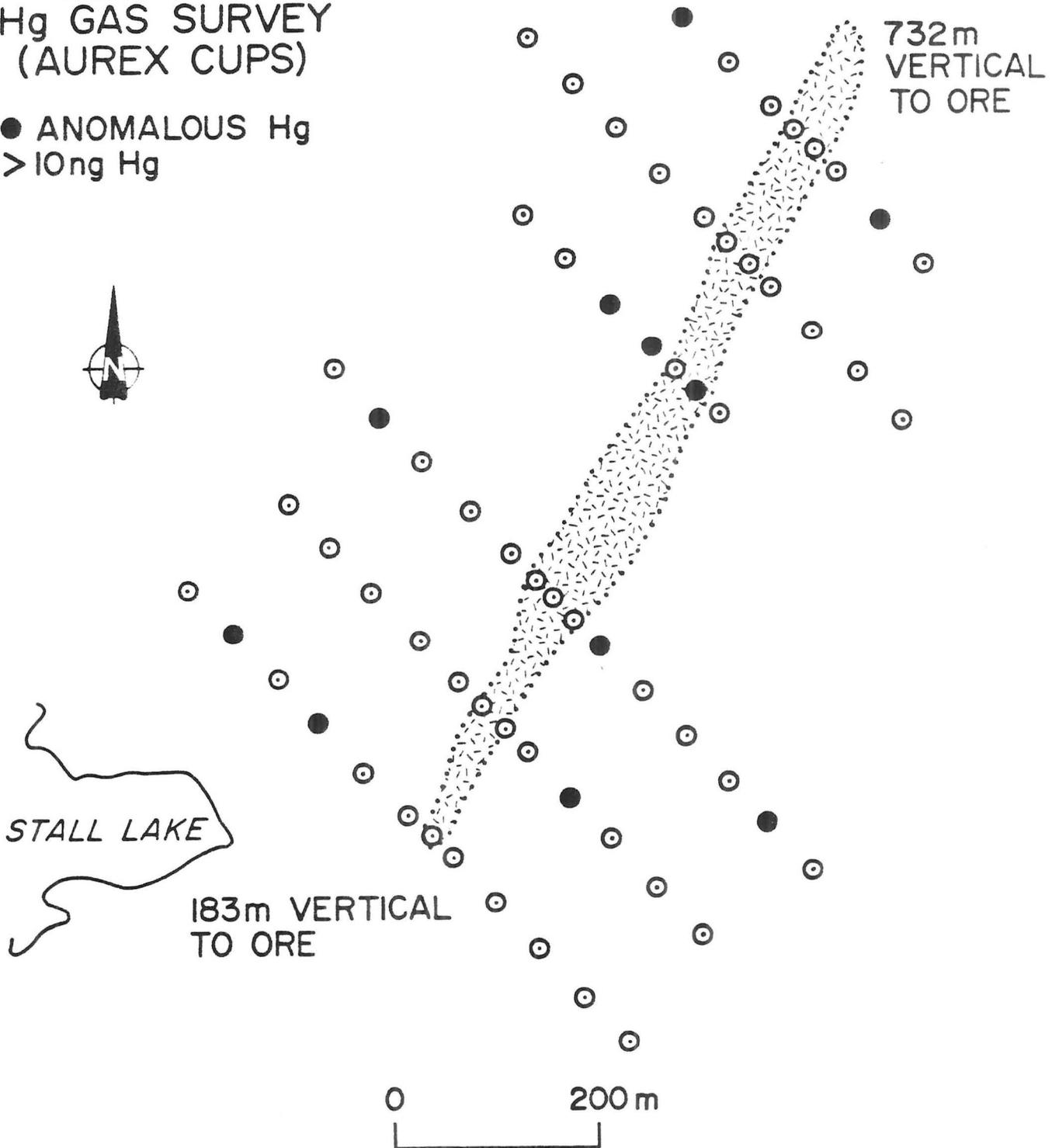
Figure 19: Results of the Rod Cu-Zn deposit mercury gas survey.
