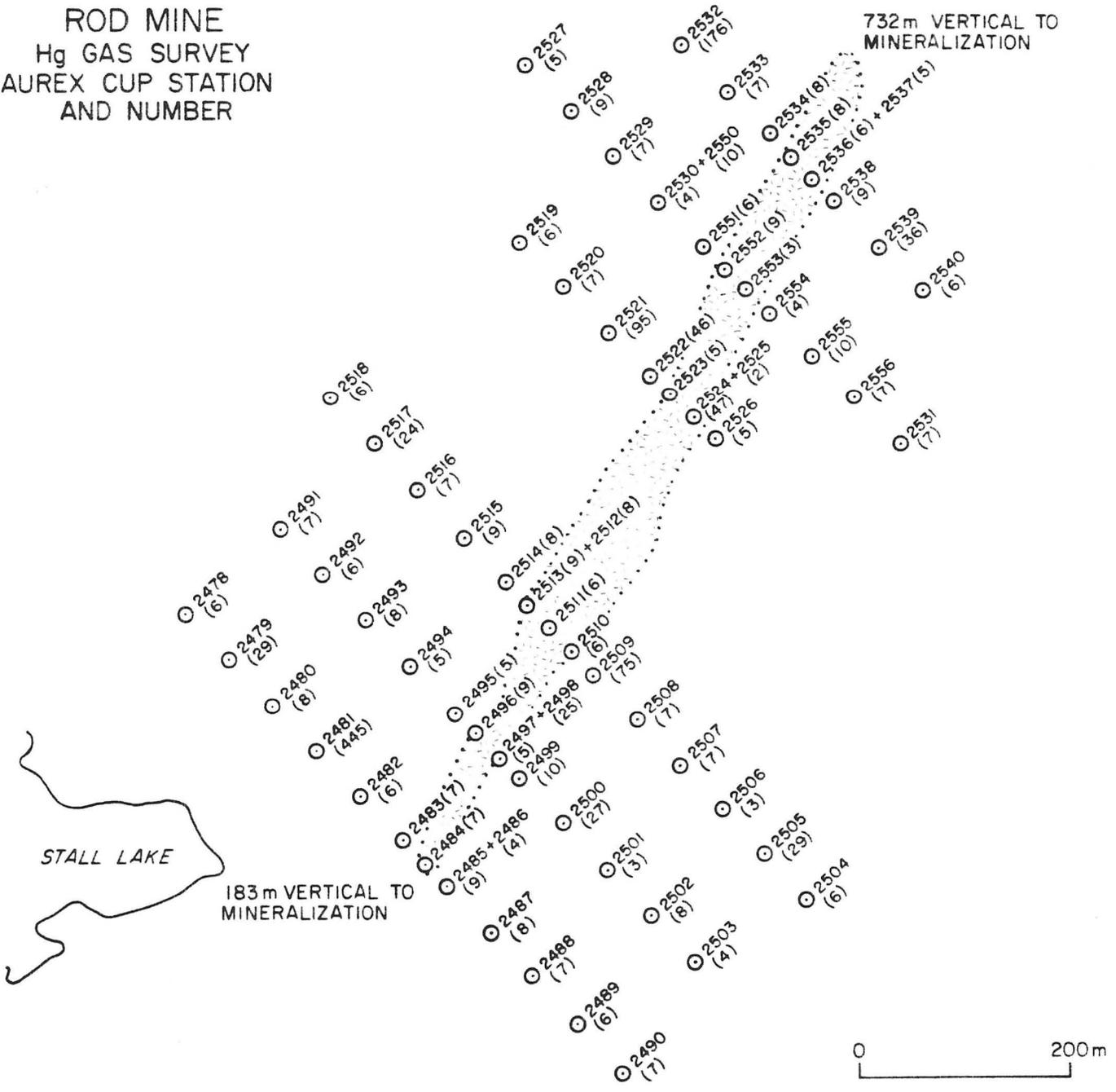
Figure 18: Location of Aurex Cups over the Rod Cu-Zn deposit, Snow Lake area. Bracketed figures represent nanograms of Hg at that station.
