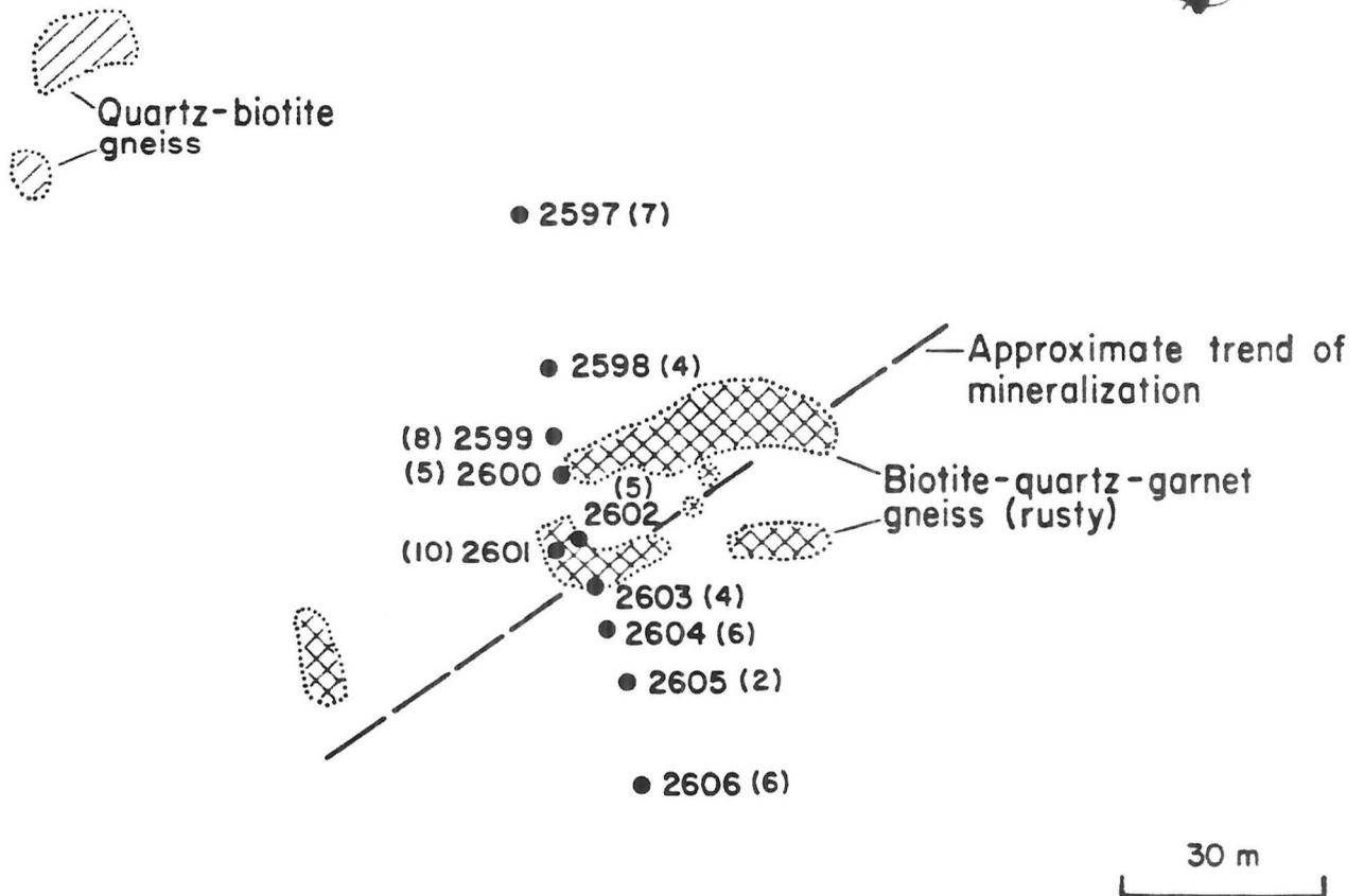
Figure 15: Results of the Kobar Pb-Ag occurrence mercury gas survey. Bracketed figure represents nanograms of Hg; 4 digit number adjacent to sample location represents the Aurex Cup number.
