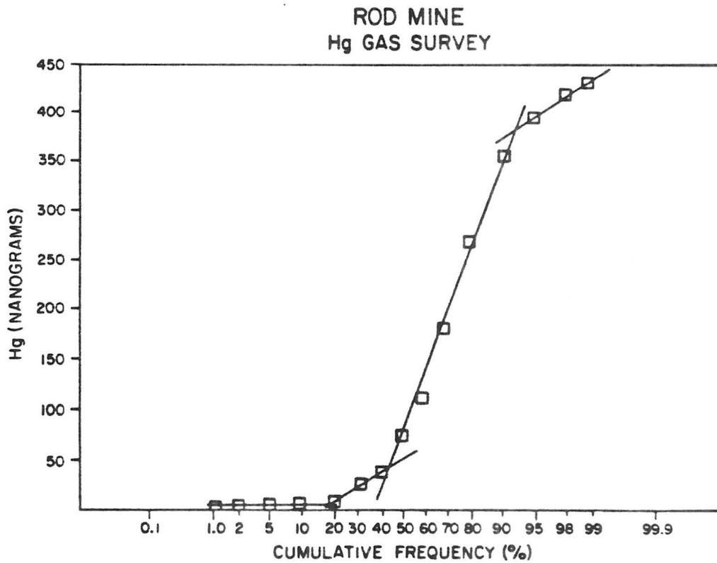
Figure 17: The cumulative frequency determination of mercury gas threshold in the Rod Cu-Zn deposit survey.
