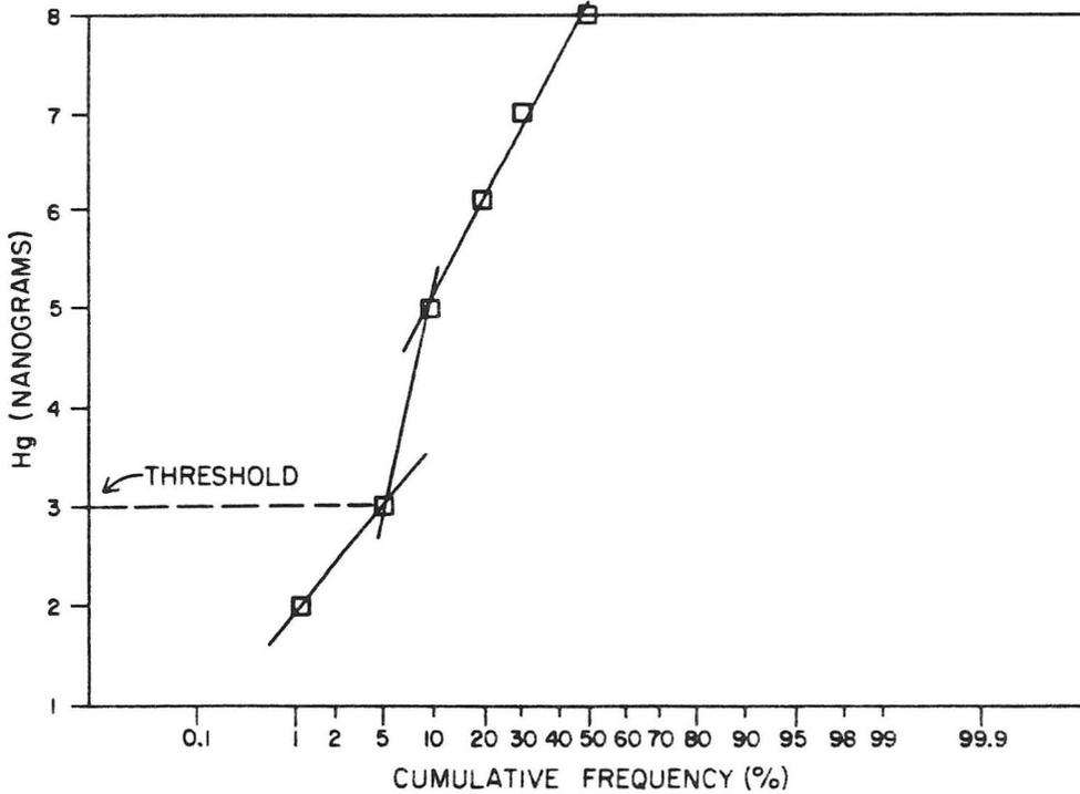
Figure 13: The cumulative frequency determination of mercury gas threshold in the Stall Lake Cu-Zn deposit survey.
