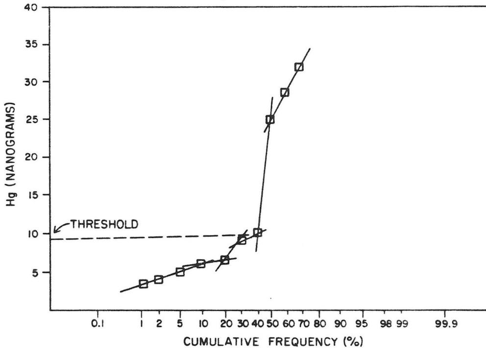
Figure 9: The cumulative frequency determination of mercury gas threshold in the Rushed Au showing survey.
