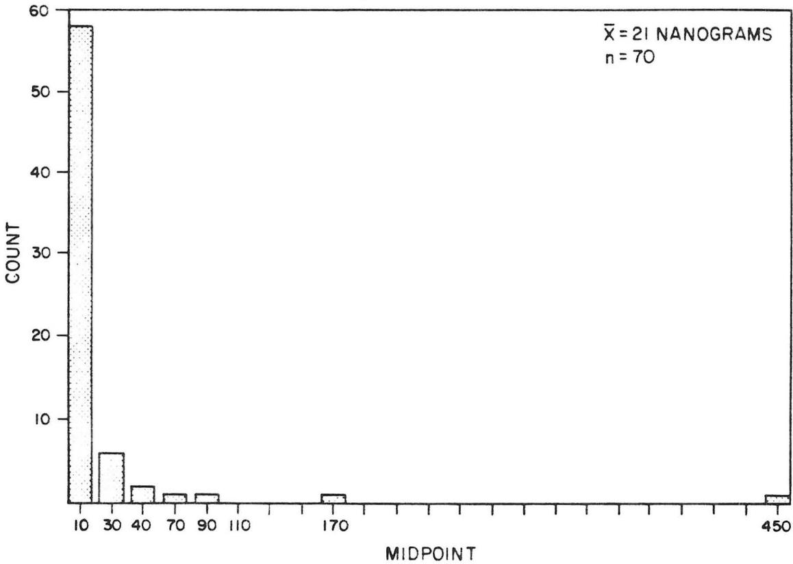
Figure 16: Mercury gas data distribution for the Rod Cu-Zn deposit, Snow Lake.
