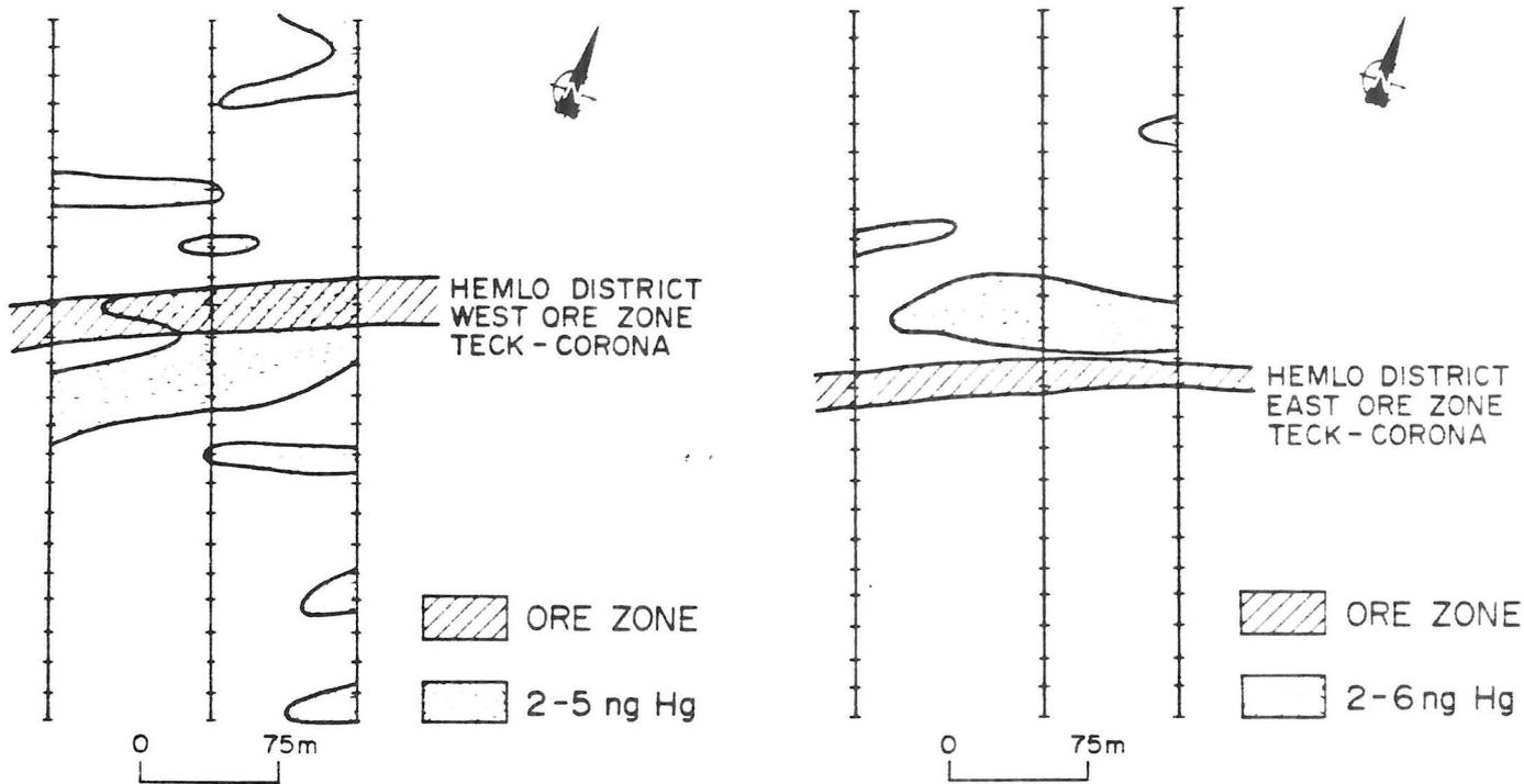
Figure 6: Results of an Aurex cup mercury gas survey at the Hemlo Au deposit, Ontario. Diagram and results from Barth Search Inc., 1985.
