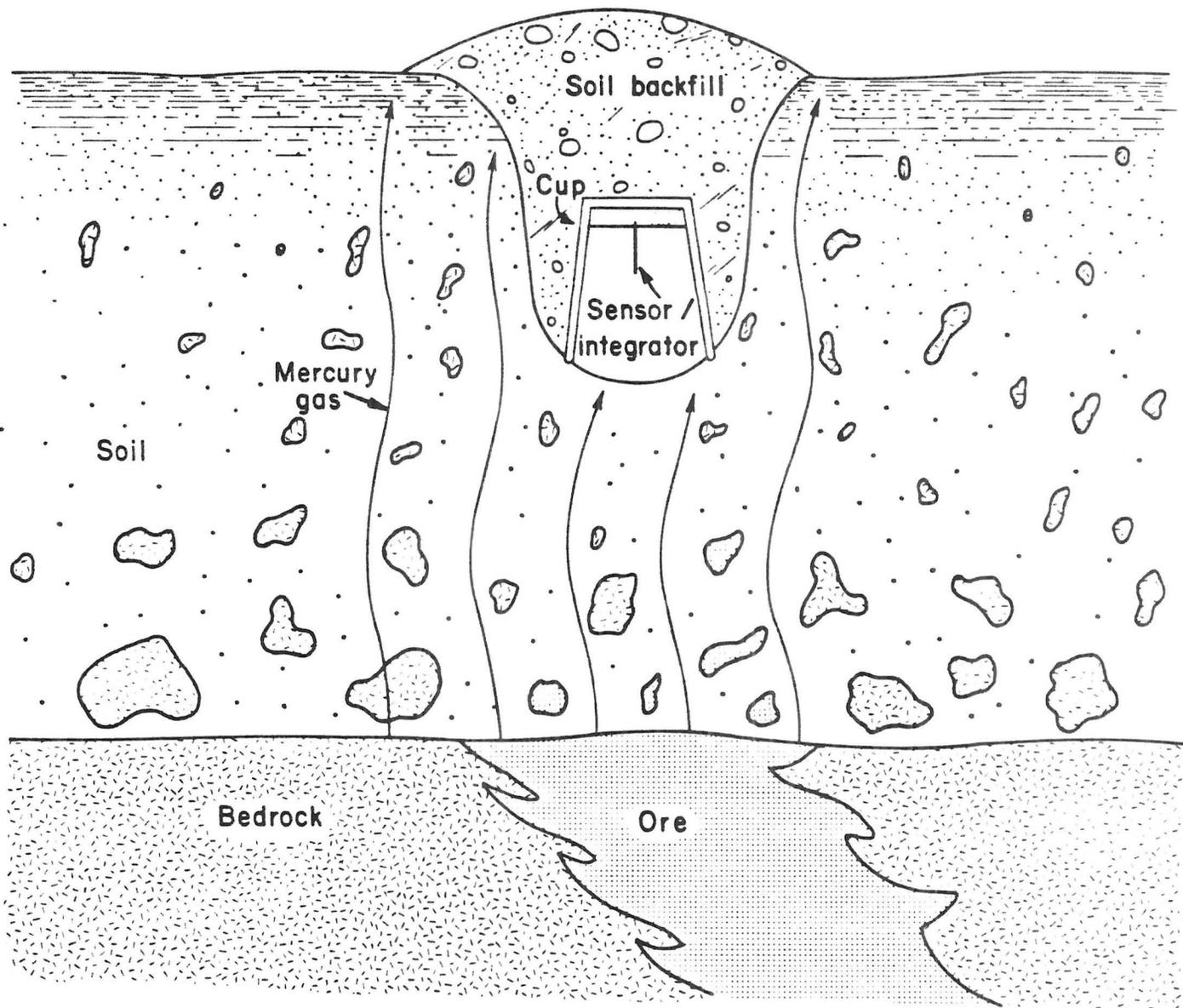
Figure 4: Schematic diagram illustrating the application of Aurex Cups in the measurement of mercury gas. Diagram from Earth Search Inc., 1985.
