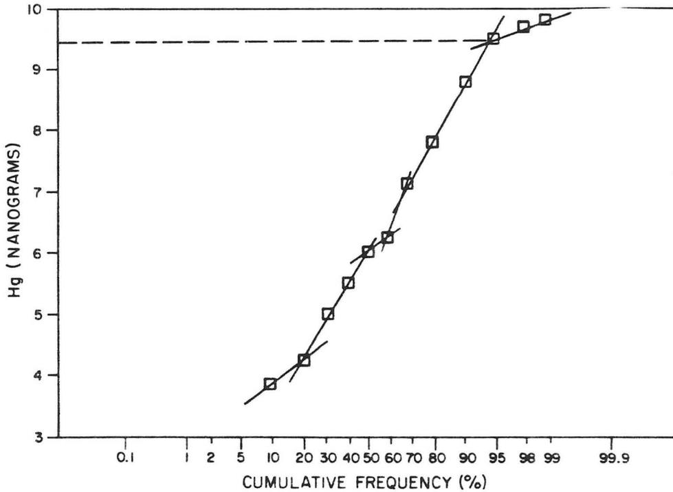
Figure 14: The cumulative frequency determination of mercury gas threshold in the Kobar Pb-Ag occurrence survey.
