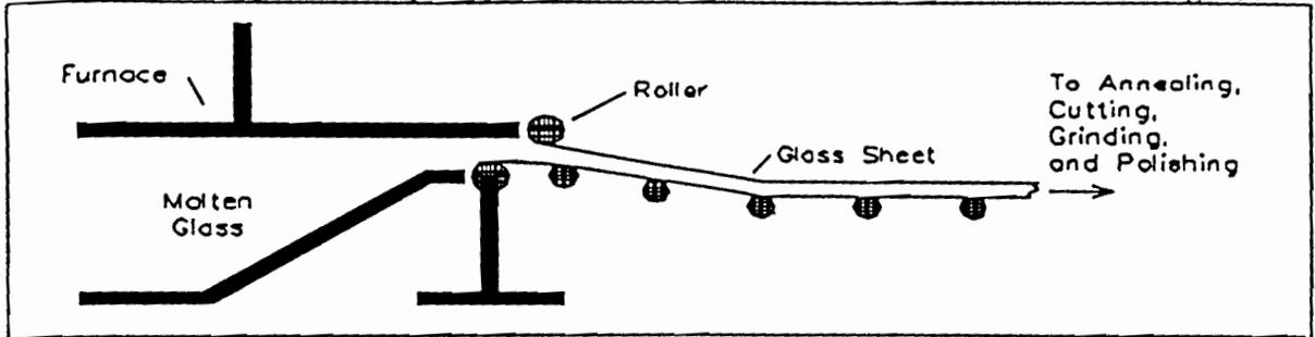
Figure 4. Simplified plate glass forming process.
