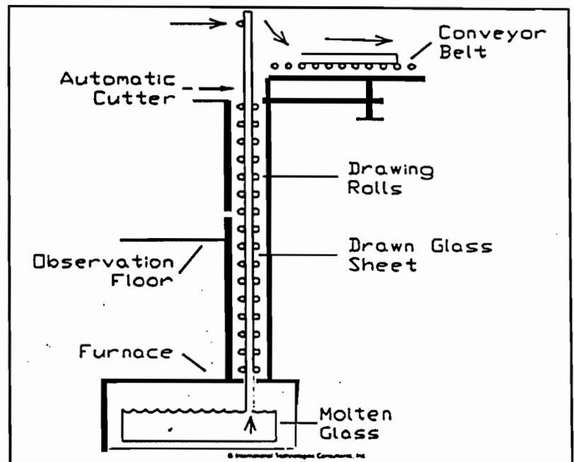
Figure 3. Simplified vertical draw sheet process.
