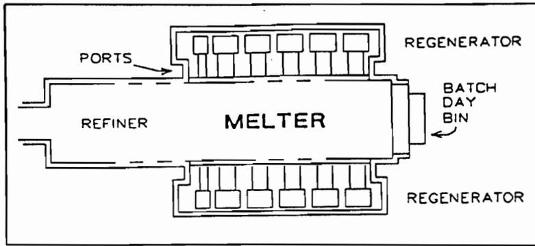
Figure 2. Typical melting furnace.
