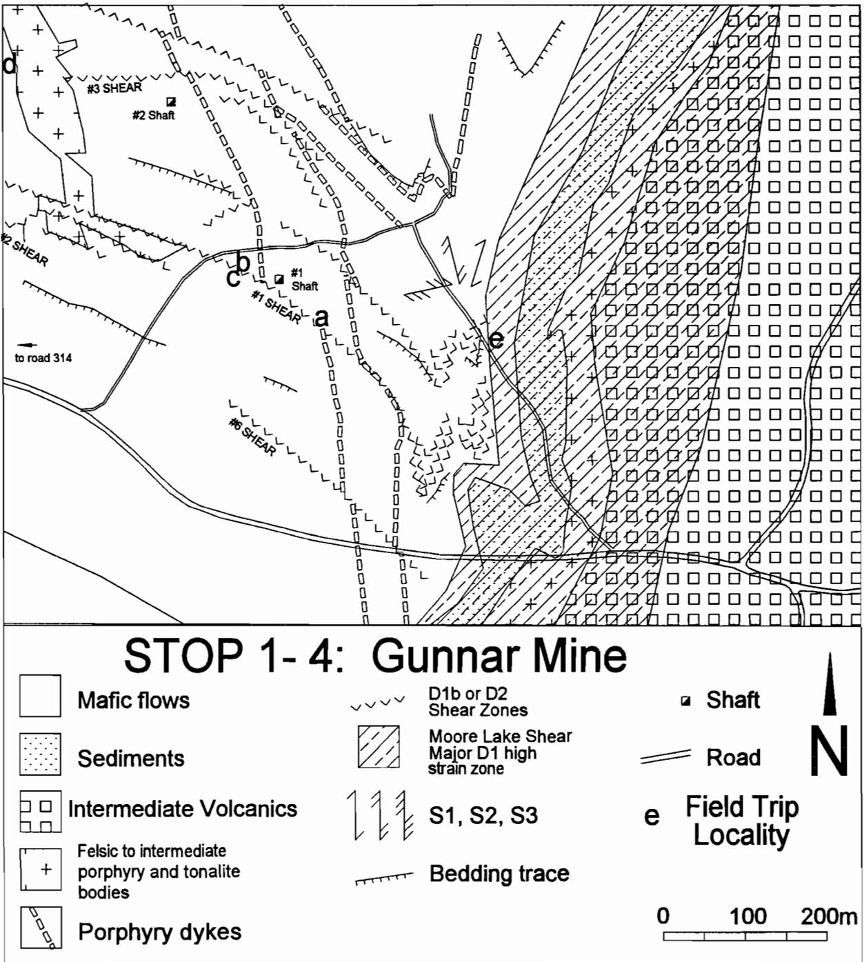
Figure 24: Geological sketch of the Gunnar Mine area (after Stockwell and Lord, 1939; Brommecker, 1991).
