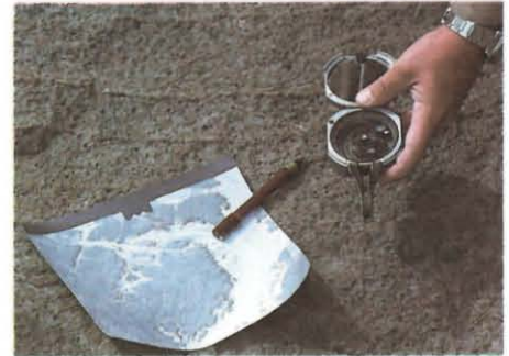
Top left: Ground electromagnetic survey. Top right: Airborne vertical gradiometer system used to measure magnetic gradient. Bottom left: Constructing a field map using a planetable. Bottom right: Compass and air photograph for orientation in bush.
