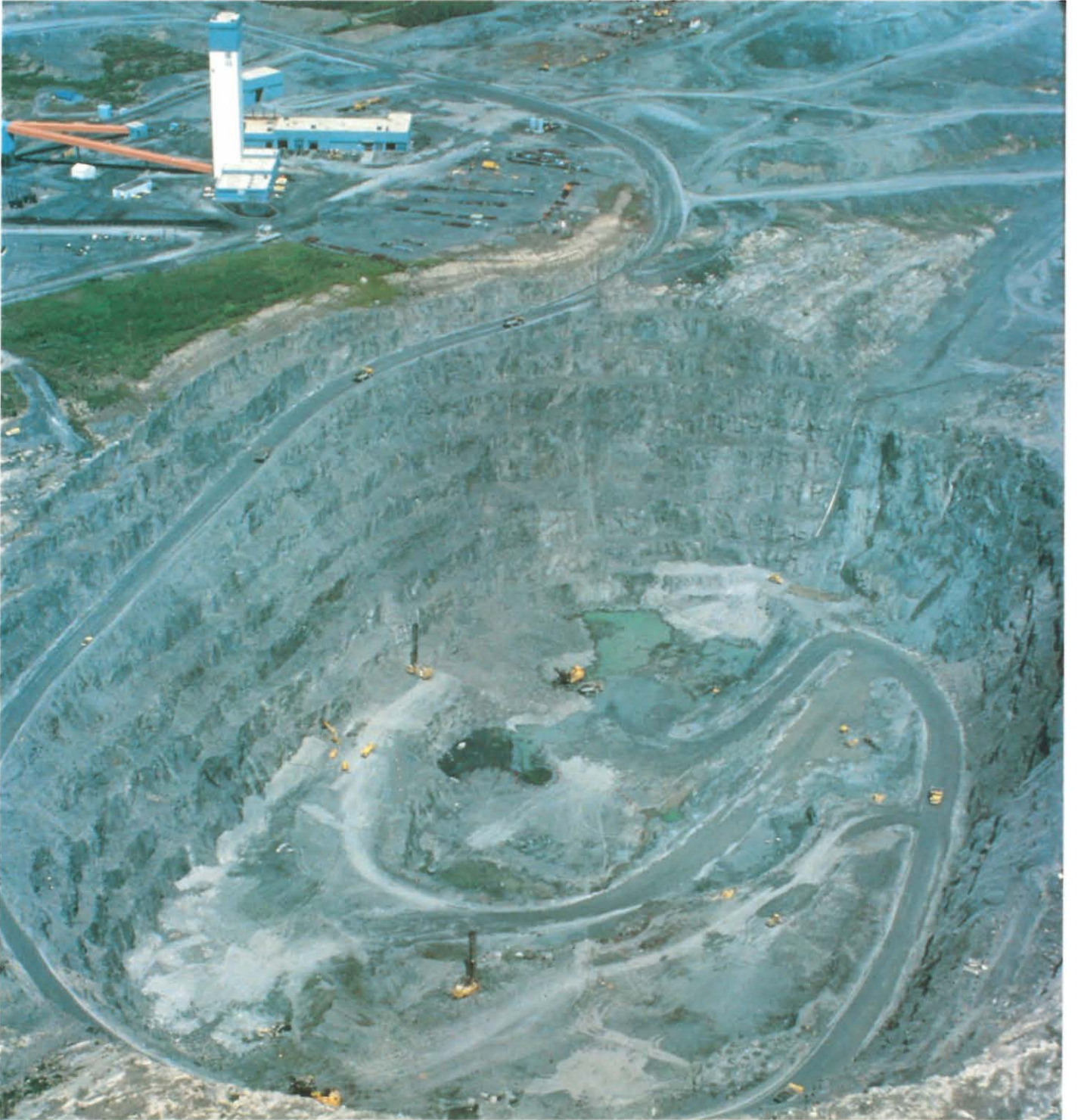
Inco Limited's Pipe Open Pit and No. 2 Headframe in background. Large steam shovels, drills and trucks are dwarfed by the size of the pit. Access road spirals upward along pit walls (circa 1980).
