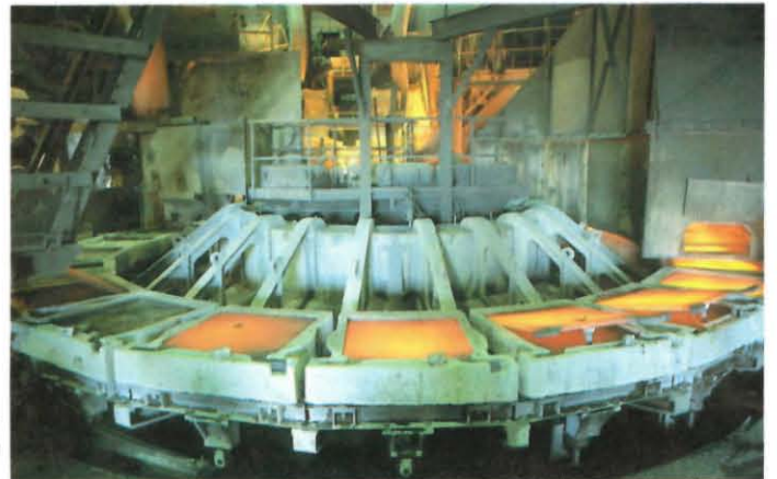
Molten copper is cast into anodes weighing approximately 240 kilograms for later transport to a refinery in Montreal.
