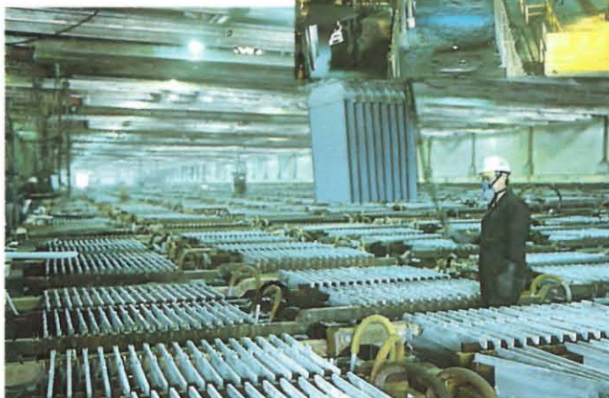
In Hudson Bay's tankhouse zinc is deposited on cathodes in 1180 electrolytic cells. A set of cathodes is being transported in the picture, 1986.
