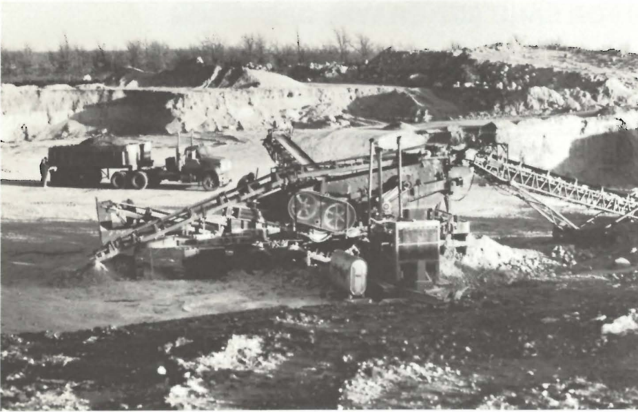
Figure 16: Portable crushing and screening operation in a gravel pit. The processed gravel is hailed to the work site by truck.
