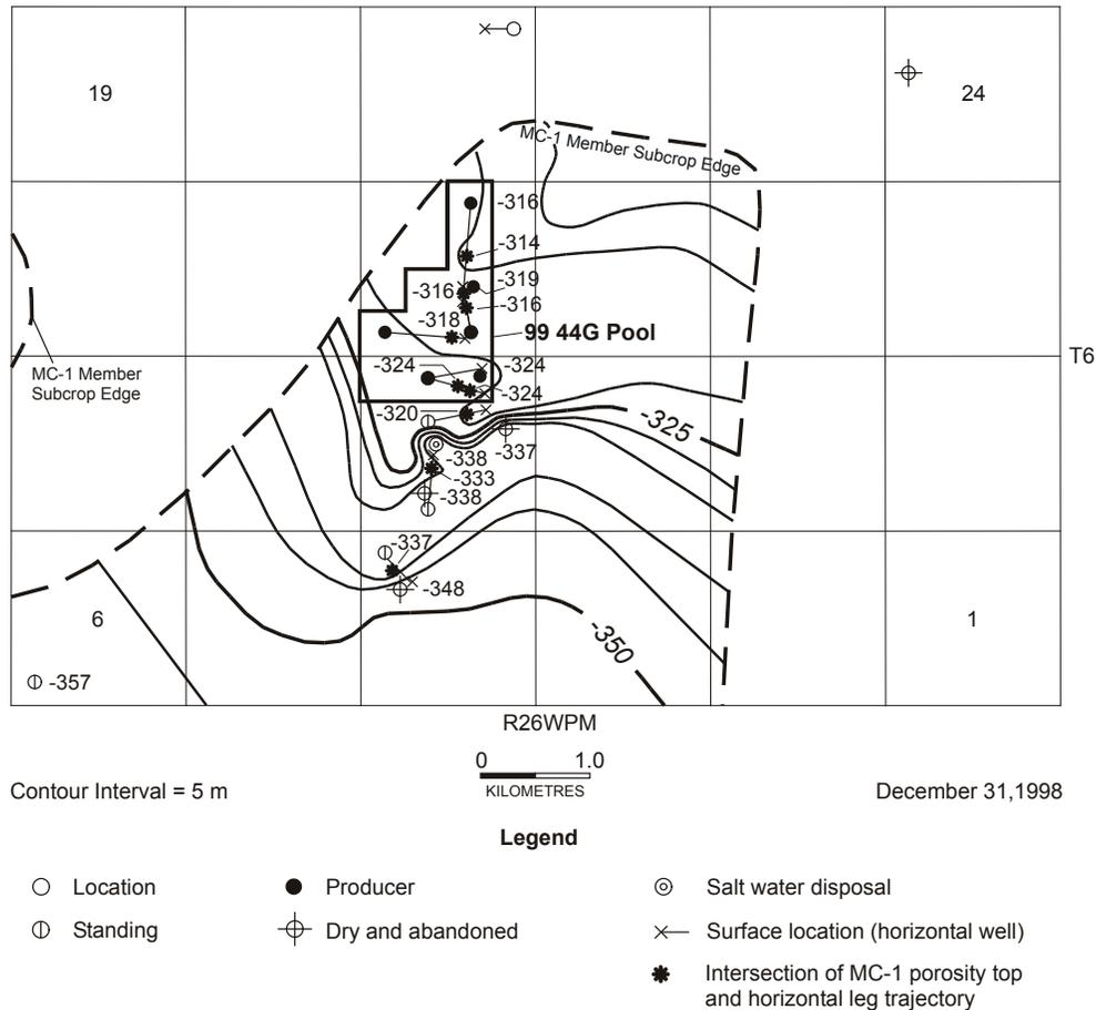
Figure 28: Structure on top of the MC-1 Member porosity, Other Areas MC-1 G Pool (99 44G), southwestern Manitoba.
