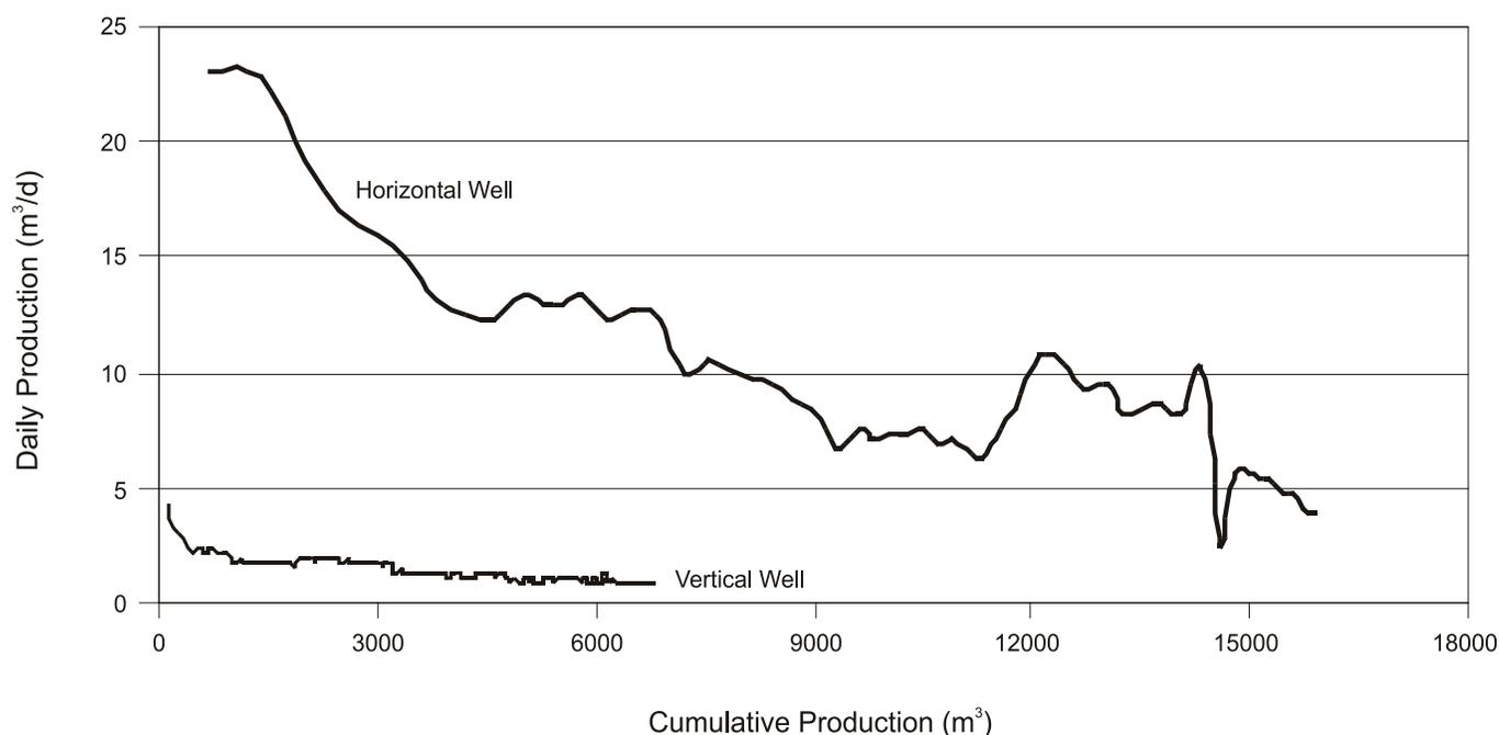
Figure 22: Comparison of vertical and horizontal well performance, MC-1 Member, southwestern Manitoba.
