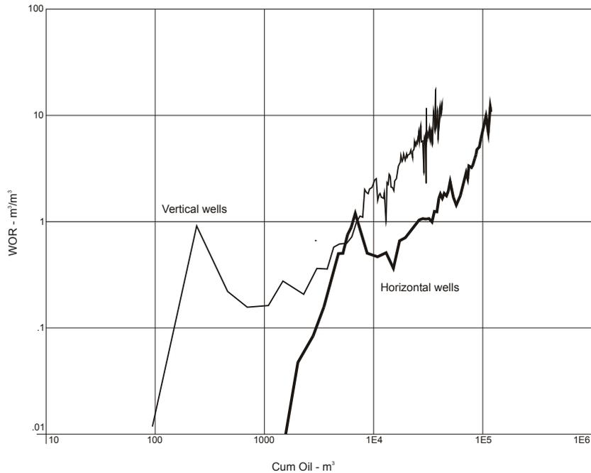
Figure 25: Comparison of water coning between vertical and horizontal wells, Tilston MC-1 C Pool (02 44C), southwestern Manitoba.
