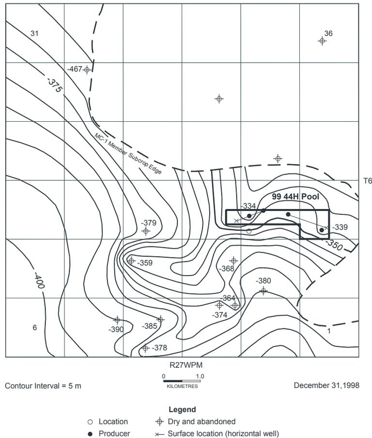
Figure 29: Structure on top of the MC-1 Member porosity, Other Areas MC-1 H Pool (99 44H), southwestern Manitoba.
