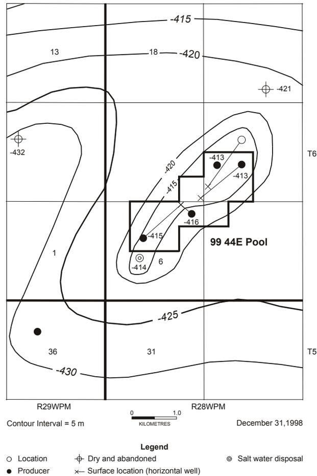
Figure 27: Structure on top of the MC-1 Member porosity, Other Areas MC-1 E Pool (99 44E), southwestern Manitoba.
