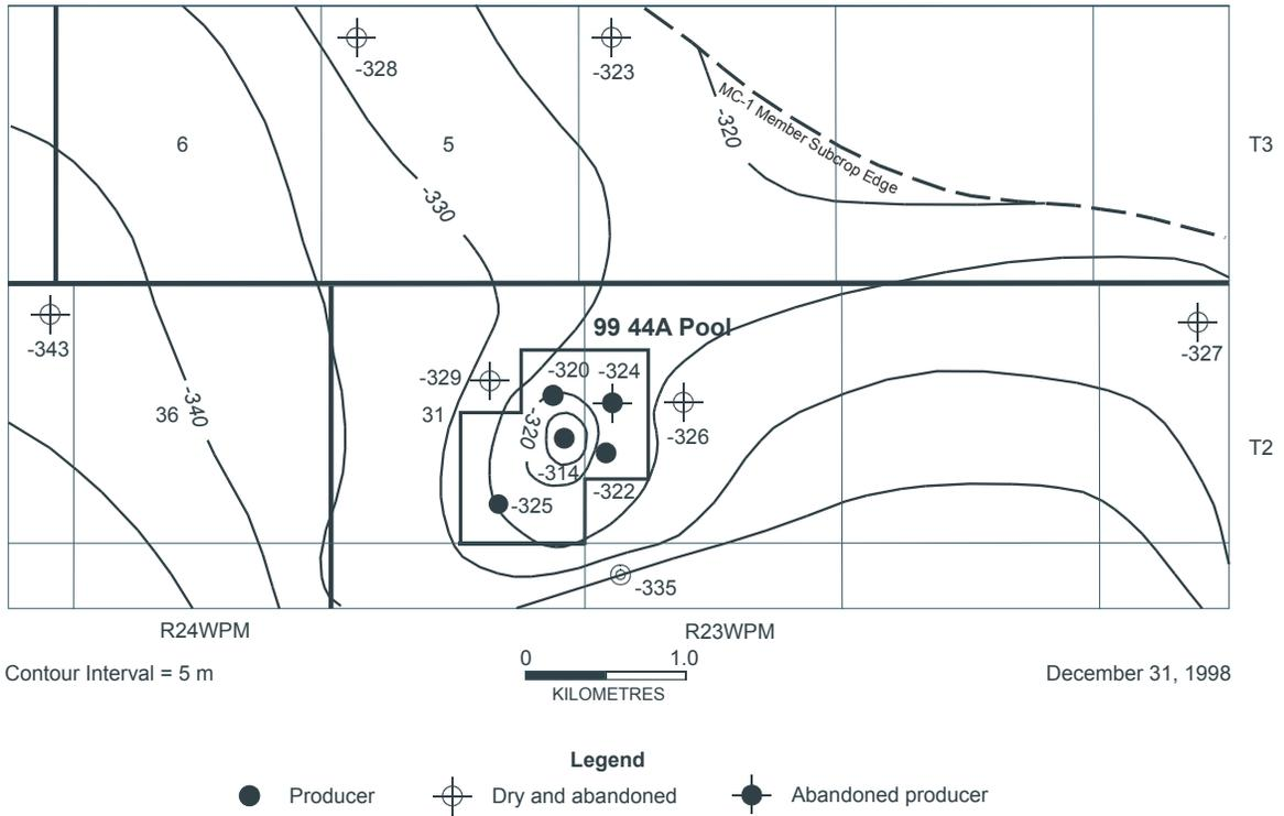
Figure 26: Structure on top of the MC-1 Member porosity, Other Areas MC-1 A Pool (99 44A), southwestern Manitoba.
