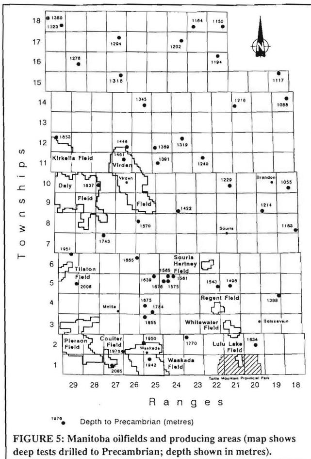
FIGURE 5: Manitoba oilfields and producing areas (map shows deep tests drilled to Precambrian; depth shown in metres).
