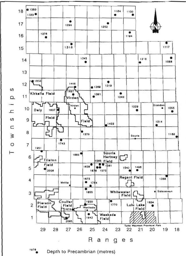
FIGURE 5: Manitoba oilfields and producing areas (map shows deep tests drilled to Precambrian; depth shown in metres).
