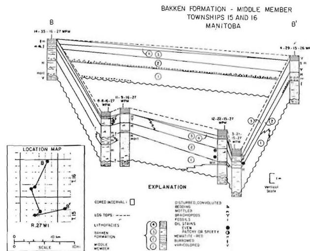
Figure 9: Fence diagram showing the distribution of the lithofacies units of the Middle Member of the Bakken Formation in Townships 15 and 16, Manitoba. Lithofacies represented are described from cores. Sedimentary features, as well as oil staining are indicated.
