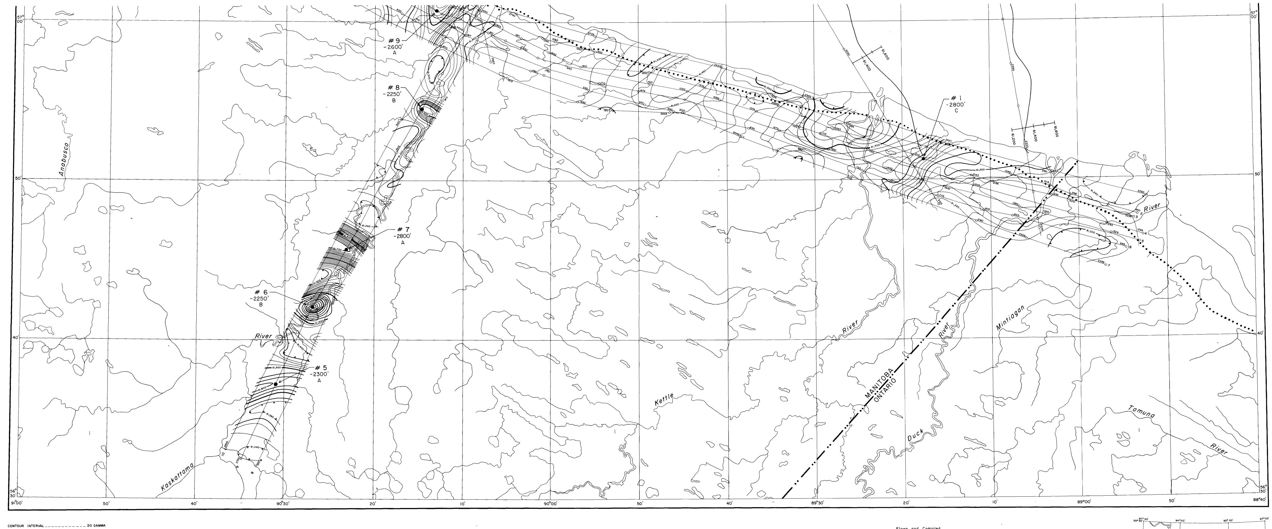
MEAN TERRAIN CLEARANCE \_\_\_\_\_IOOO FEET 500 GAMMA CONTOUR\_\_\_\_\_ 100 GAMMA CONTOUR\_\_\_\_\_ 20 GAMMA CONTOUR\_\_\_\_\_ MAGNETIC LOW\_\_\_\_\_ FIDUCIAL POINTS\_\_\_\_\_ 3690 O FLIGHT LINES\_\_\_\_\_
