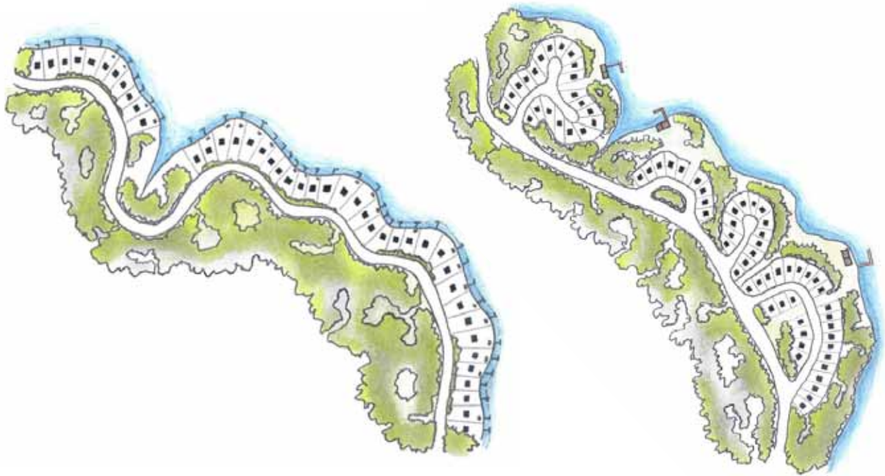
Figure 2: Common (left) vs. recommended (right) subdivision design
