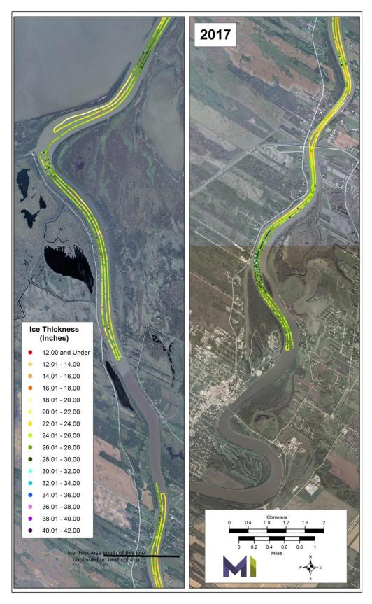
$Figure\ 10-Ice\ Thickness\ Measurements\ based\ on\ Ground\ Penetrating\ Radar,\ Red\ River\ North$
