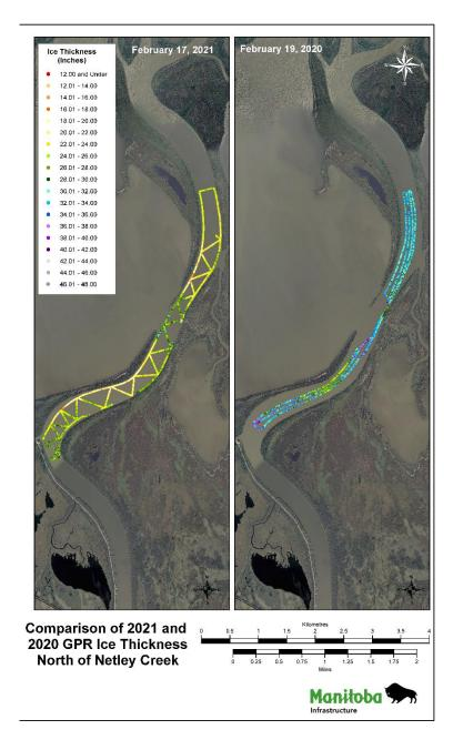
Figure 13 – Ice Thickness Measurements (inches) based on Ground Penetrating Radar: Red River (2020 vs 2021)
