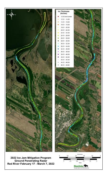
Figure 12 – Ice Thickness Measurements (inches) based on Ground Penetrating Radar: Red River 2022.
