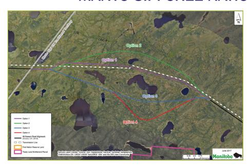
Manto Sipi Cree Nation initially identified an alignment near the community that was parallel to the winter road that crossed through a large bog/fen. Sourcing the necessary rock to construct an approximate 8 km segment along the winter road would require additional access roads and quarries. Manitoba Infrastructure proposed three alternative options to reduce the project footprint, cost and construction timelines.
