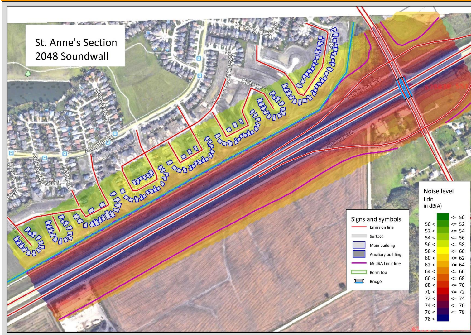
Figure A26 – PTH100 Sound Level 2048 – St. Anne's Section with Berm and Sound wall
