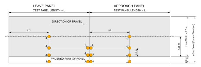
Point  $J_1$  shall be located at the centre of the panel length along the mid lane.
