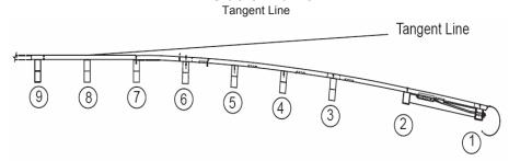
The SRT-350 8 POST<sup>TM</sup> system offsets are measured at a tangent line from the start of the SRT-350 8 POST<sup>TM</sup> system. If an offset places a post on the shoulder, then the face of the rail must be on the edge of the shoulder for that offset.
