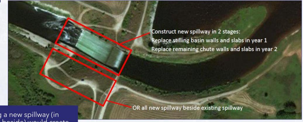
• Creating a new spillway (in place or beside) would create more capacity for water to pass through.
