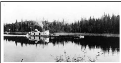
Figure 39. Stern-wheeler with ore barge on Schist Lake (Courtesy of the Public Archives of Canada PA-17233).
