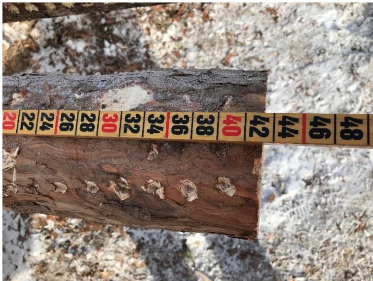
Figure 5 Length class determination in 2 cm class
