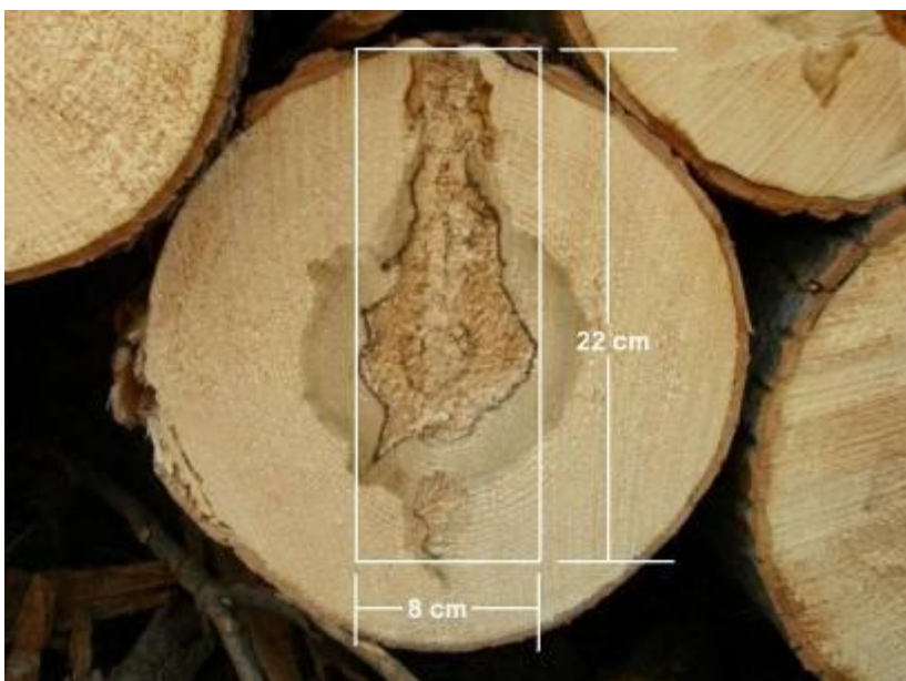
Figure 23 Long narrow defect that measures 22 cm x 8 cm
