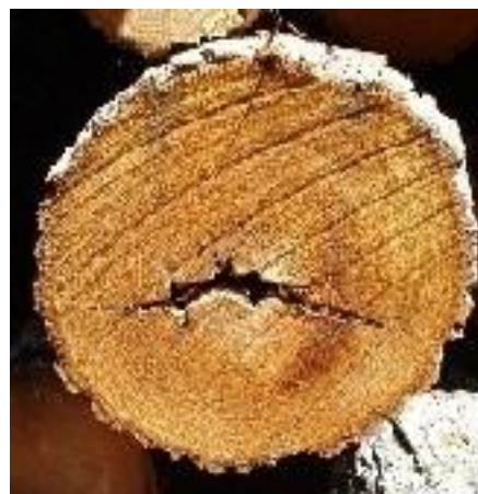
Figure 24 Heart check on the end surface of a log
