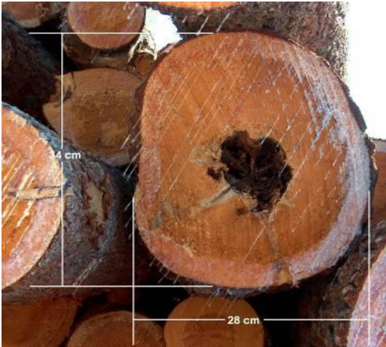
Figure 3 Measuring diameters: logs with irregular sawn surfaces
