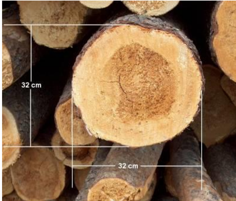
Figure 2 Measuring diameters: logs with regular sawn surfaces
