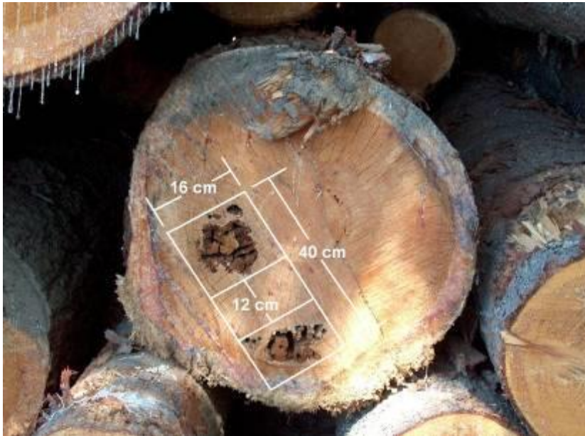
Figure 25 Two defects separated by 14 cm or less
