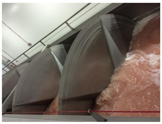
Photo 5: Cecure used to sterilize birds during chilling process.
