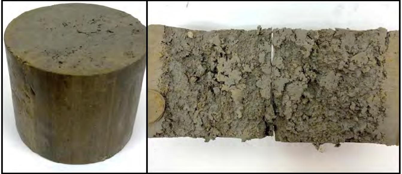
PHOTOGRAPH #1: TH, 3'-5' after hydraulic conductivity testing.
