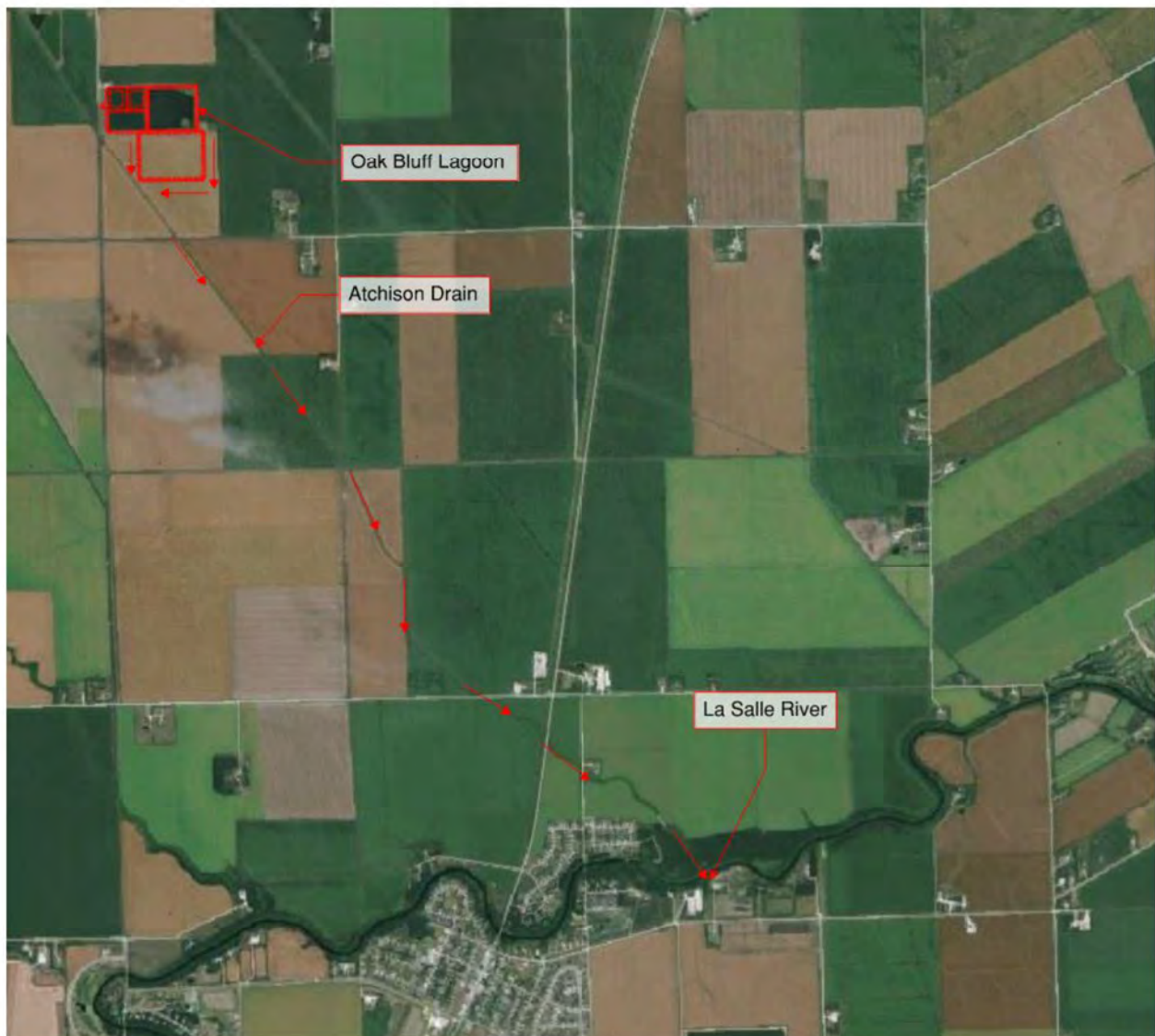
Figure 5-1: Proposed Effluent Discharge Route
