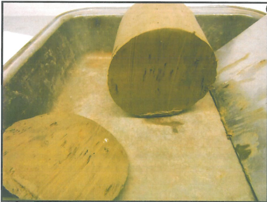
PHOTOGRAPH #6: Sample #S7 after breaking apart.
