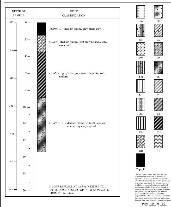
Past JRCC Test Hole Logs
