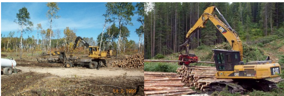
Figure 6.18 Slasher (left) slashes tree-length logs into 2.5 m bolts, a processor head on an excavator (right) performs the same task.
