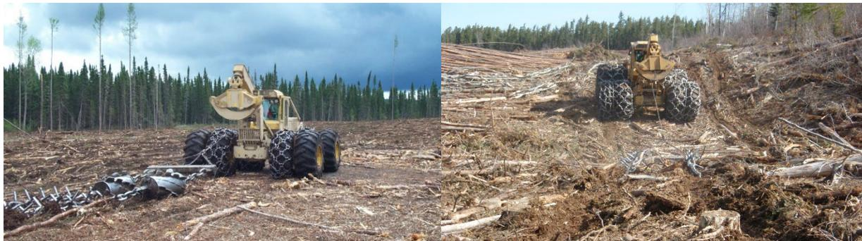
**Figure 5-7: Site preparation of a cutover using shark-fin barrels and anchor chains.**
