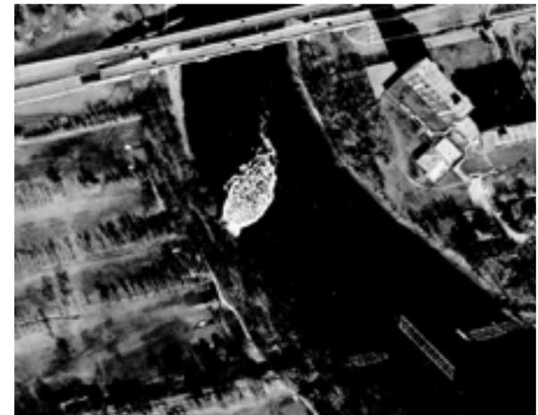
Figure 6: A plume from the North End Pollution Control Centre extends into the Red River south of the Chief Peguis Bridge.
